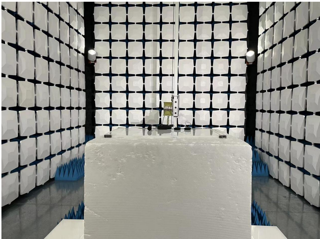
Above 1GHz for radiated emission test setup
