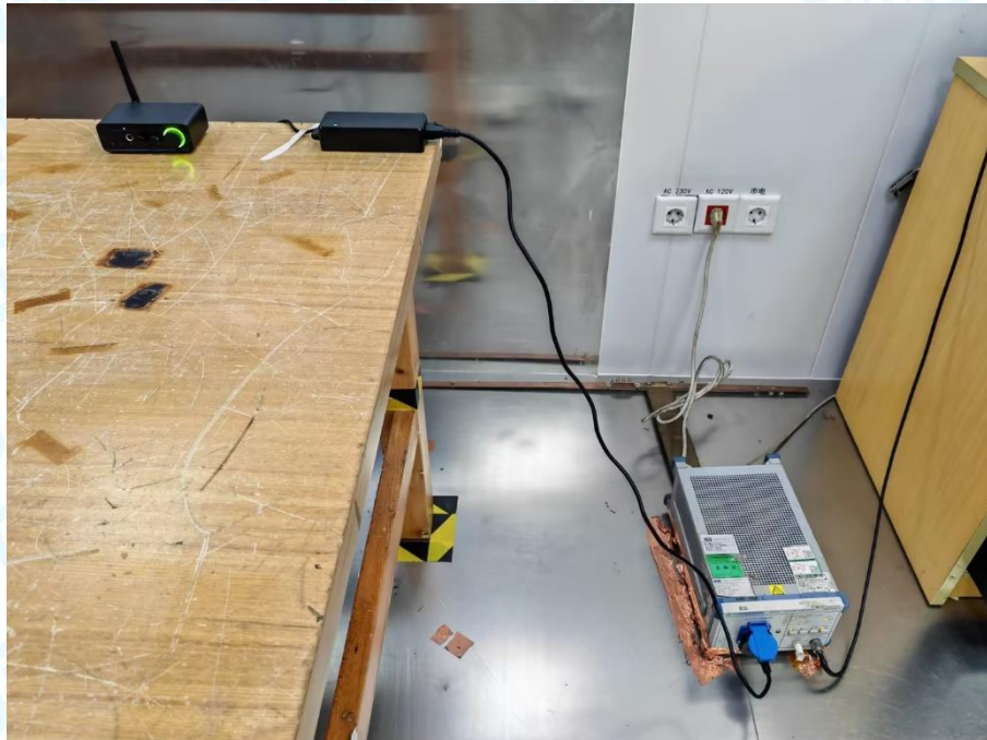
Photo of Setup for Radiated Emission (30MHz~1GHz)
