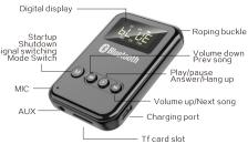
M: Long press it 3s to start/close the machine, single click it to switch modes, double click it to switch signals Long press it to reduce volume, short press it to select the previous song
