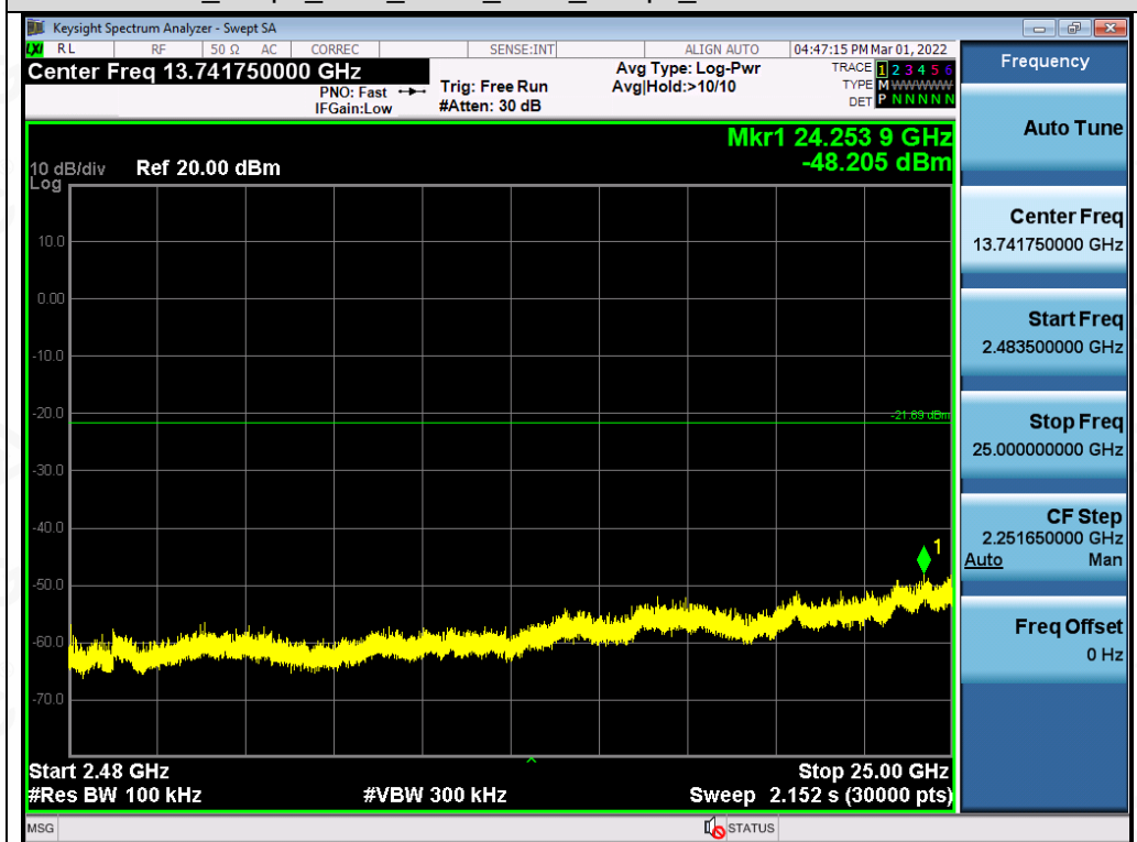
Test_Graph_EDR_ANT1_2441_3Mbps_Higher Band Emissions
