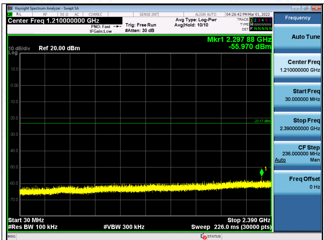
Test_Graph_EDR_ANT1_2402_2Mbps_Lower Band Emissions
