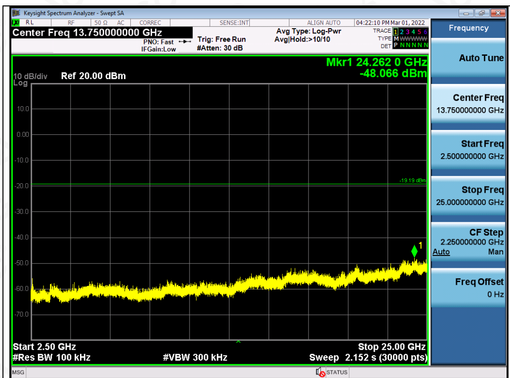
Test_Graph_BR_ANT1_2480_1Mbps_Higher Band Emissions
