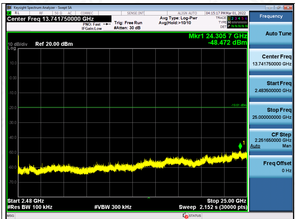
Test_Graph_BR_ANT1_2402_1Mbps_Higher Band Emissions
