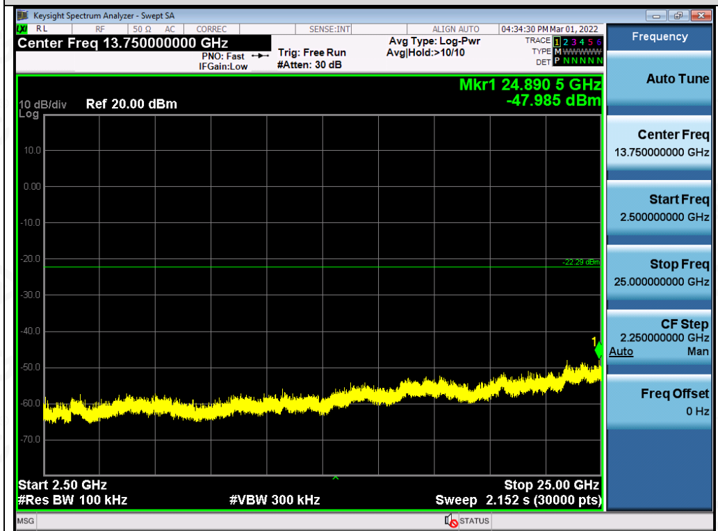
Test_Graph_EDR_ANT1_2480_2Mbps_Higher Band Emissions
