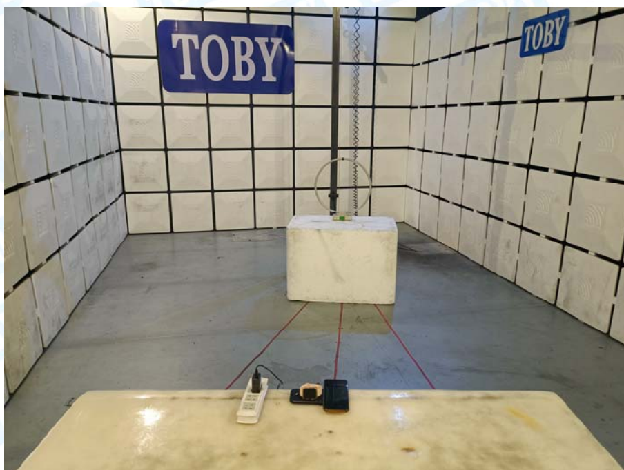
Photo of Setup for Radiated Emission (9KHz-30MHz)
