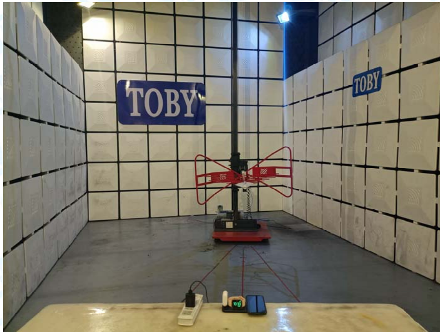
Photo of Setup for Radiated Emission (9KHz-30MHz)
