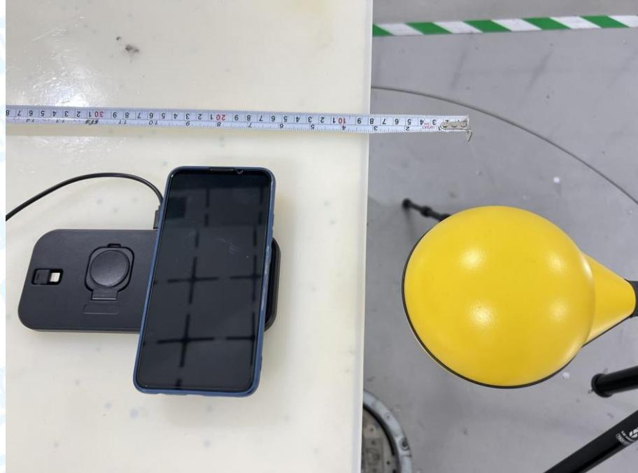
**H-Field Strength- 15 cm****Test Position E - Exposure photo from top surface**
