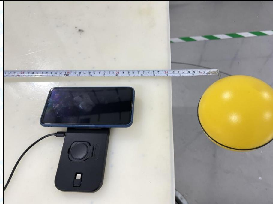
**H-Field Strength-15cm****Test Position A - Exposure photo from side edge surface-Rear**
