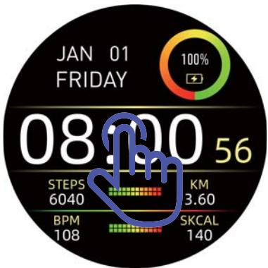
f. Power ON/OFF: Long press power button for 3s to power on; From home page, long press power button 3s, and tap/✓ to power off.
