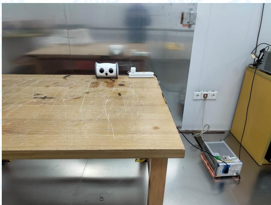
Photo of Setup for Conducted Emission
