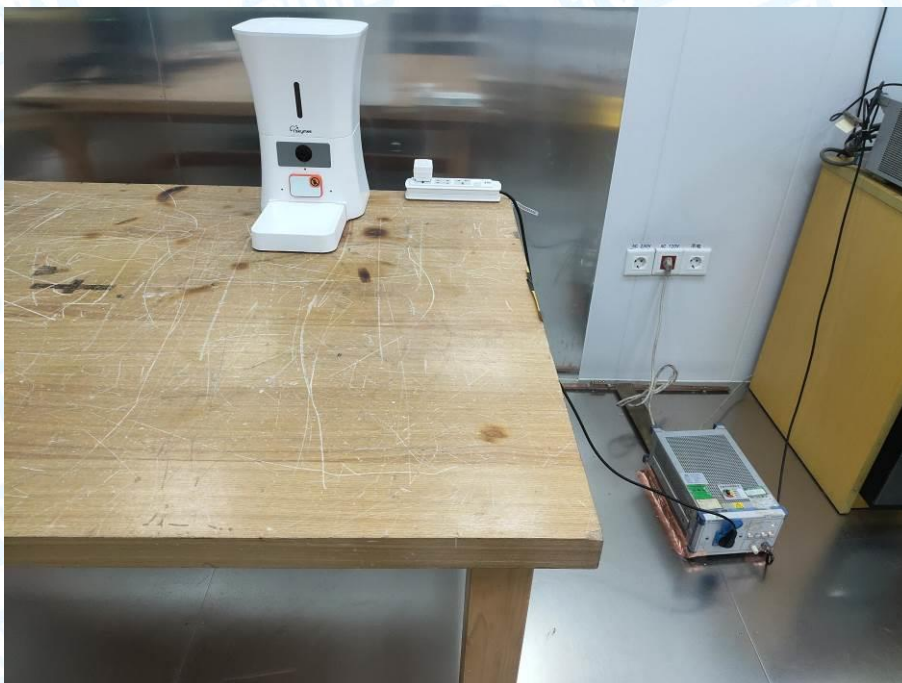
Photo of Setup for Conducted Emission
