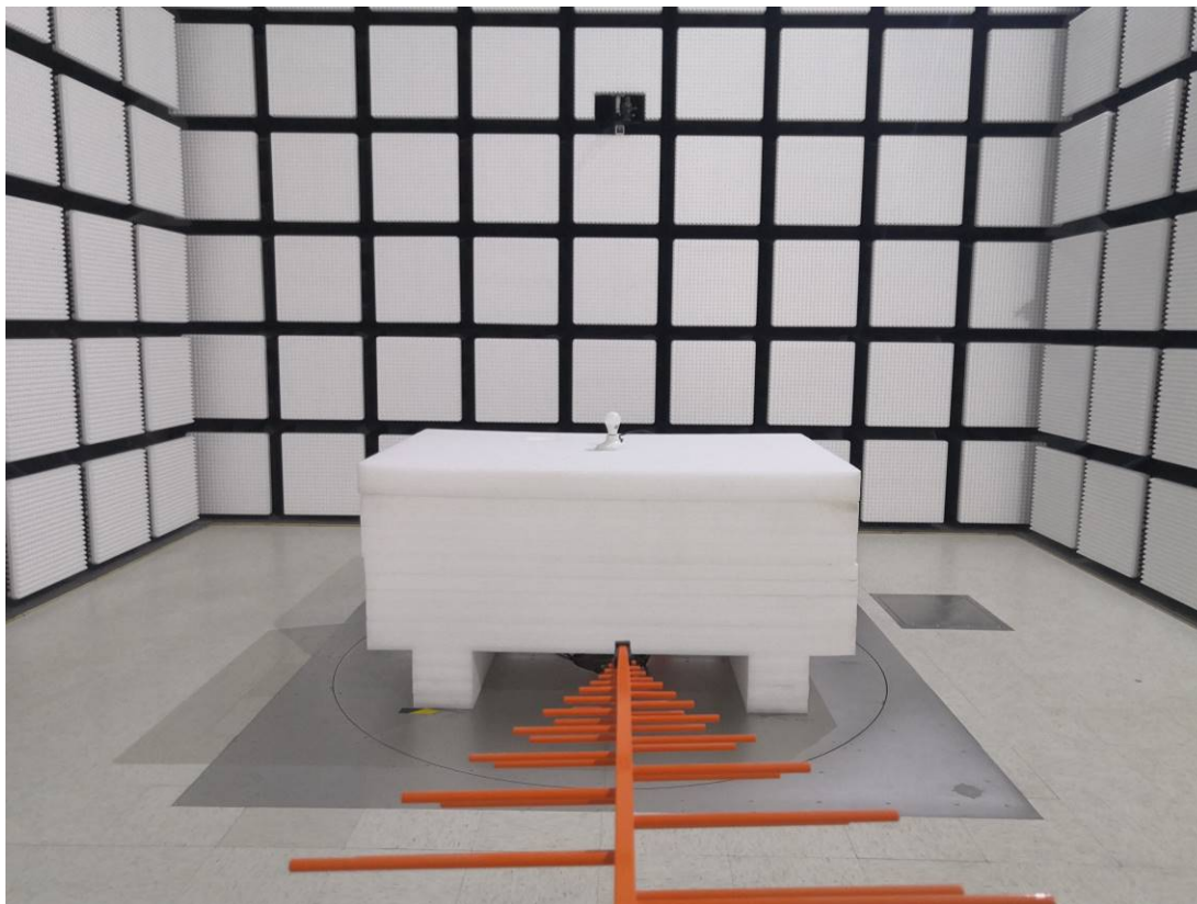
Radiated Emission Above 1GHz View
