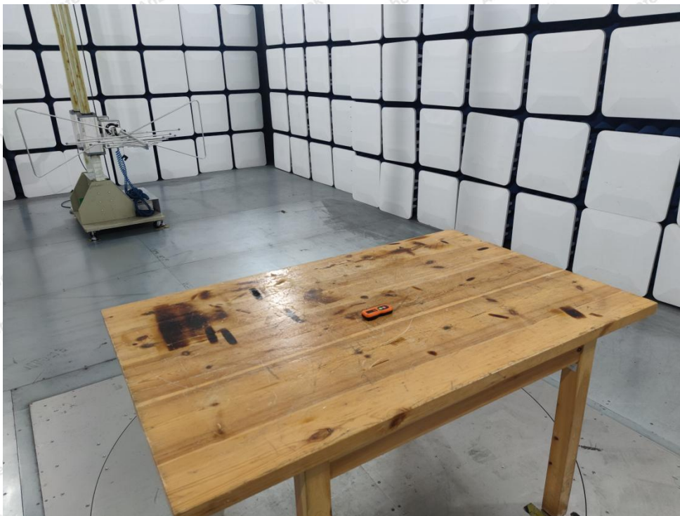
Photo of Radiation Emission Test
