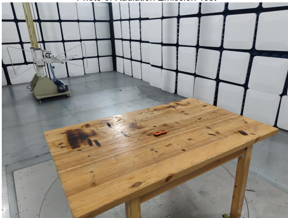
Photo of Radiation Emission Test
