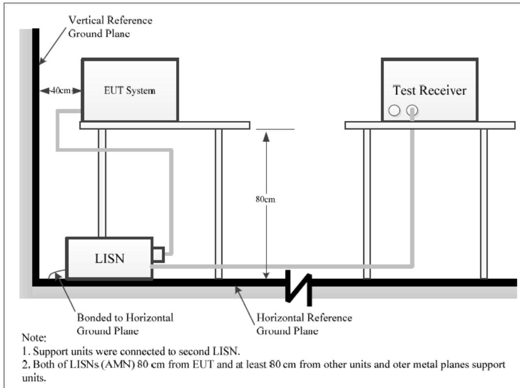
The measurement procedure of EUT setup is according with ANSI C63.10-2013. The related limit was specified in FCC Part 15.207.
