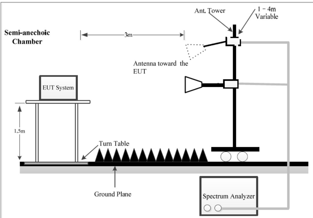
The radiated emission tests using the setup accordance with the ANSI C63.10-2013. The specification used was the FCC 15.209, and FCC 15.249 limits.
