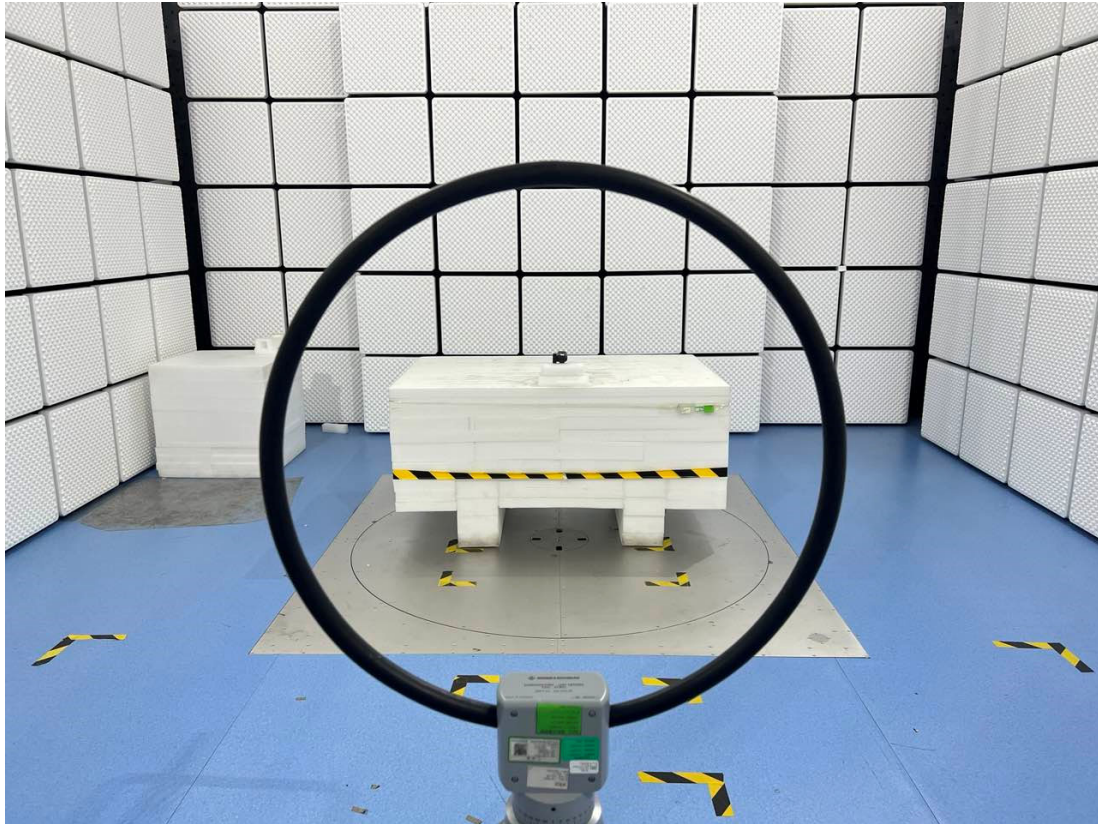
Radiated Emission - Front View (30MHz-1GHz)
