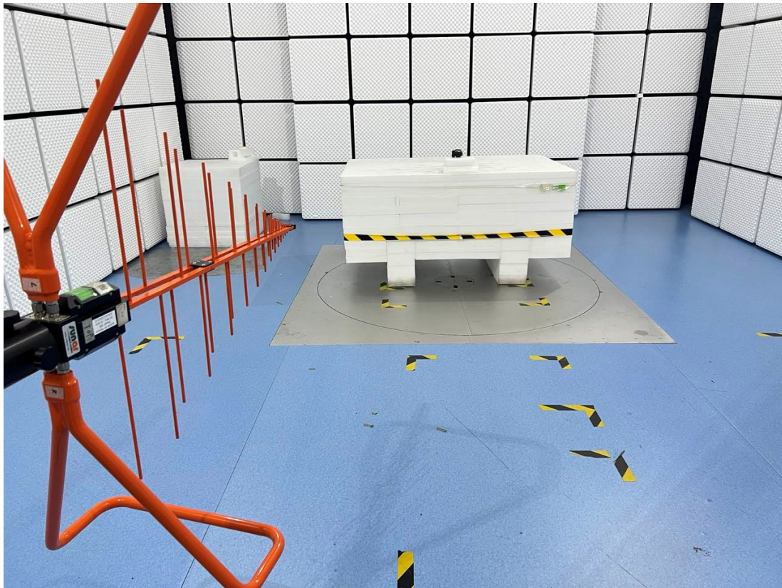
Radiated Emission - Front View (1GHz – 18GHz)
