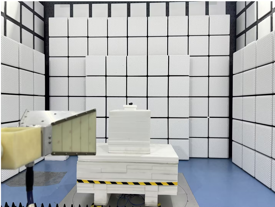
Radiated Emission - Front View (18GHz – 25GHz)
