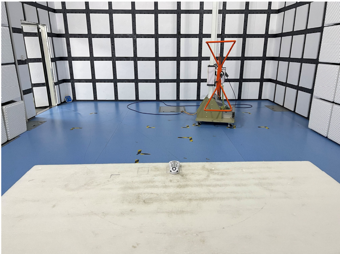
Radiated Emission - Front View (30MHz-1GHz)
