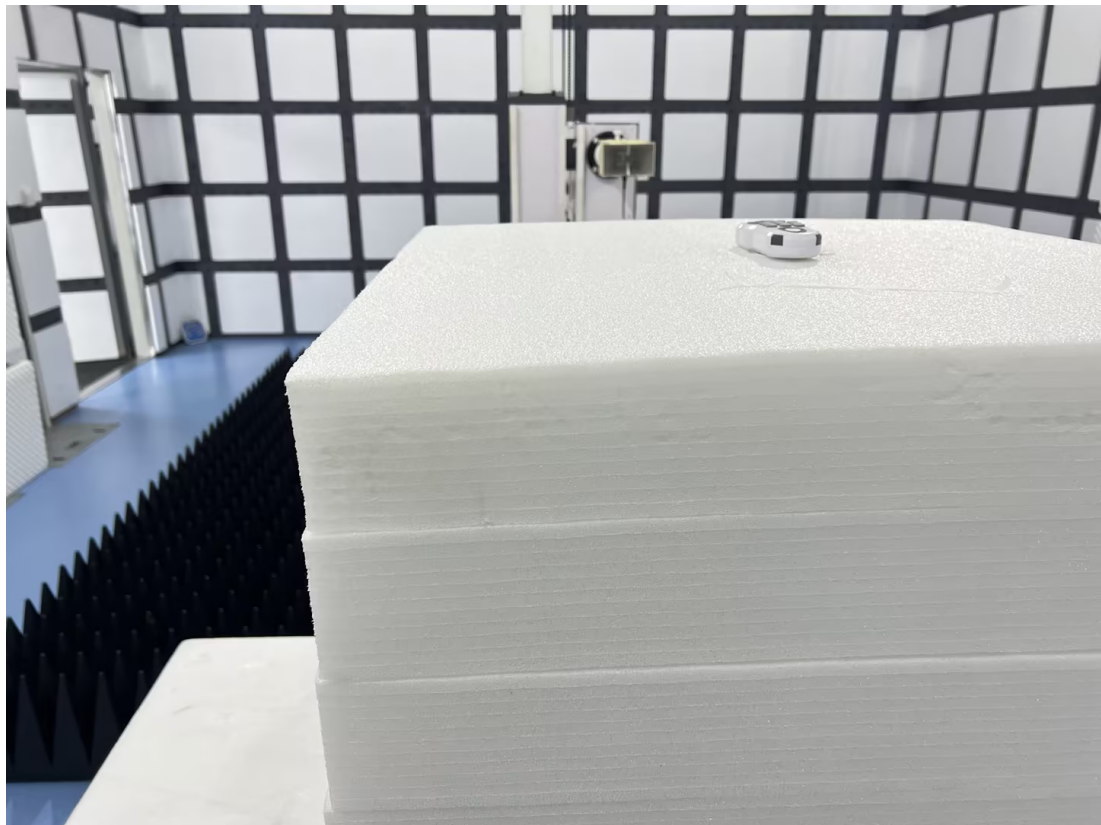
Radiated Emission - Front View (18GHz – 25GHz)
