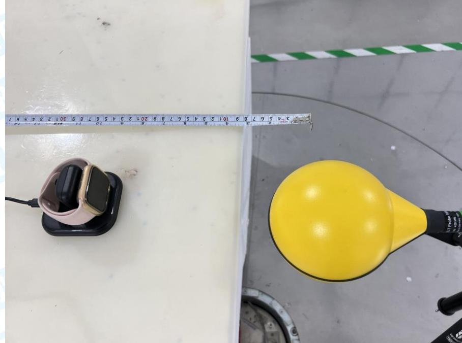
**H-Field Strength-15cm****Test Position A - Exposure photo from side edge surface-Rear**
