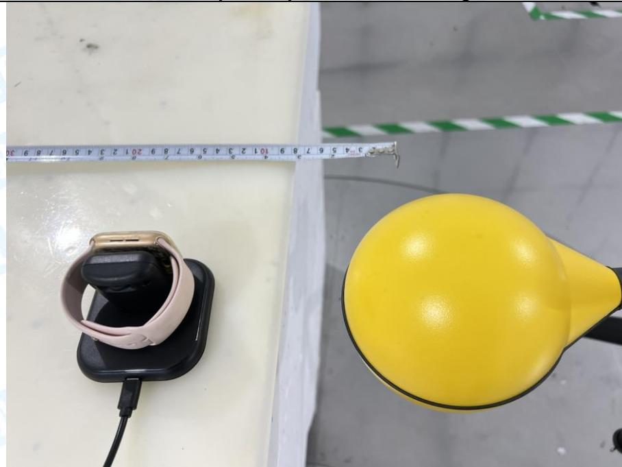
**H-Field Strength-15cm****Test Position C - Exposure photo from side edge surface-Front**
