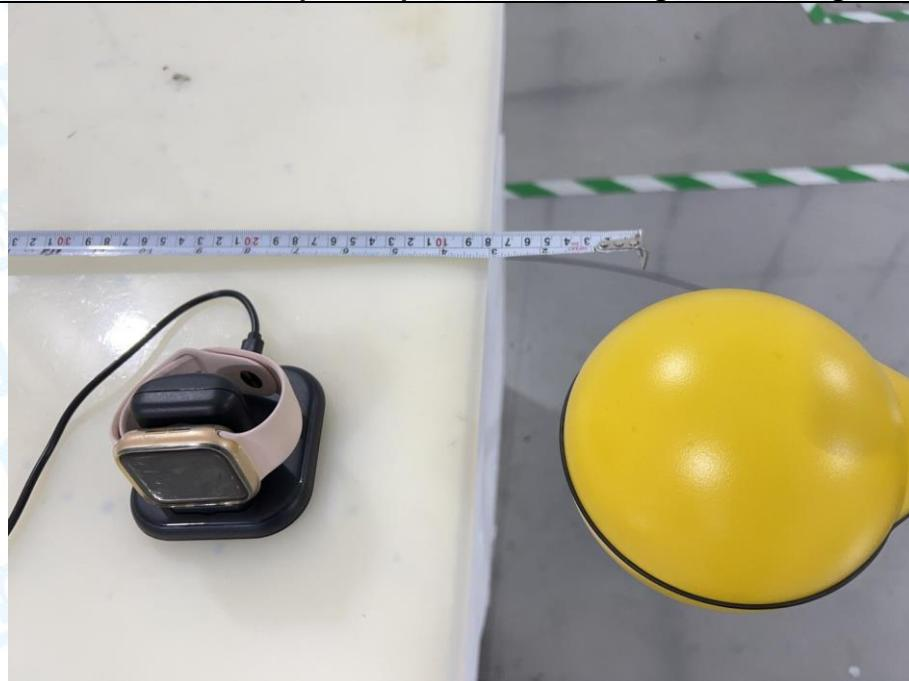
**H-Field Strength- 15 cm****Test Position E - Exposure photo from top surface**
