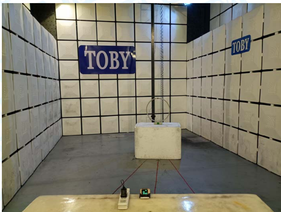
Photo of Setup for Radiated Emission (9KHz-30MHz)
