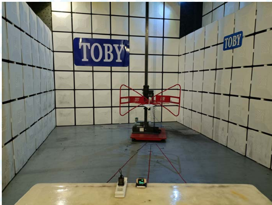
Photo of Setup for Radiated Emission (9KHz-30MHz)
