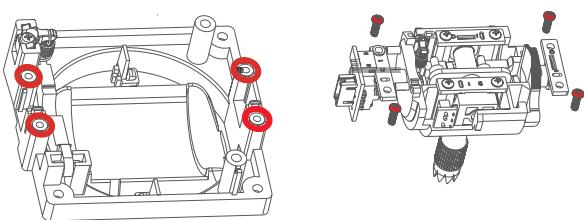
2. Loosen the screws shown in fig.4 and remove the plates.
