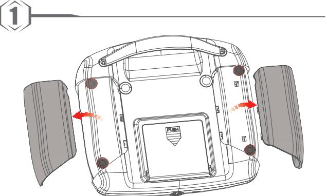
1. Use tweezers to remove the left and right hand grips. Then use a screwdriver to remove the 4 screws marked in red.
