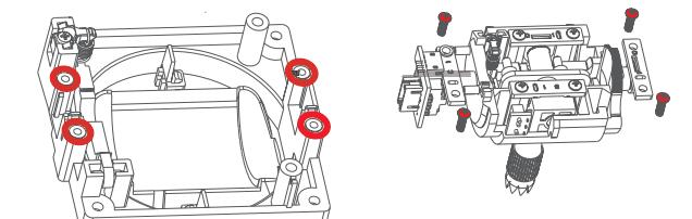
3. Loosen the assembly screws shown in fig.4 and remove the plate. Be careful to ensure no damage to cables.
