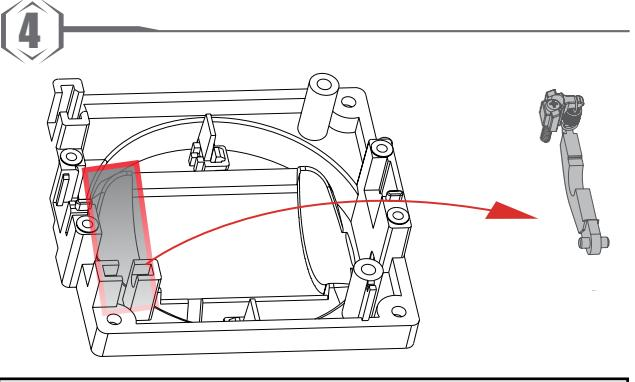
4. Remove the bottom of the seat assembly of the spring hook assembly.
