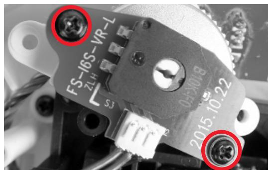
2. Remove the PCB screws marked in red.
