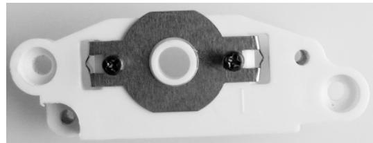
3. Remove the knob from the potentiometer and put them in a safe place.
