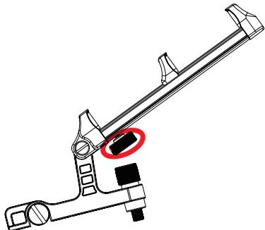
1. To adjust the bracket, loosen locking screw by turning it anti-clockwise.
