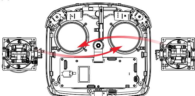
2. Swap the gimbals and rotate them 180 degrees, then line them up with the screw holes and replace the screws. (There is no need to disconnect the cables.)
