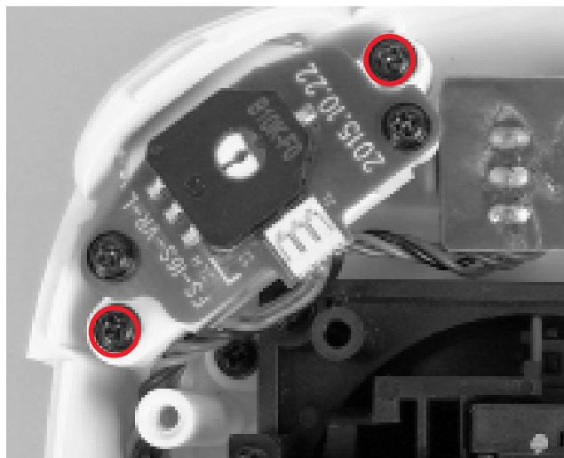
1. Take the transmitter apart, then use a screwdriver to remove the screws marked in red.
