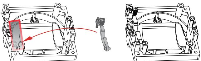
4. Place the spring hook assembly into position and hook the spring onto the hook located inside the transmitter.
