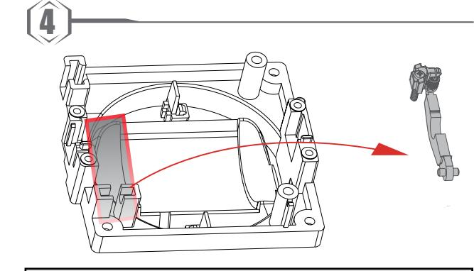
4. Remove the bottom of the seat assembly of the spring hook assembly.
