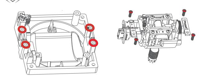
3. Loosen the assembly screws shown in fig.4 and remove the plate. Be careful to ensure no damage to cables.
