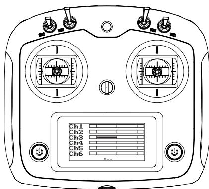
4. Turn on the transmitter and enter the servo display screen to make sure everything is working as expected.
