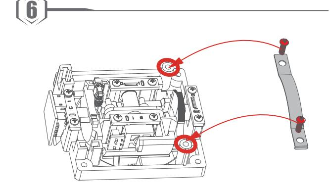
6. Secure the bracket using the screws provided.
