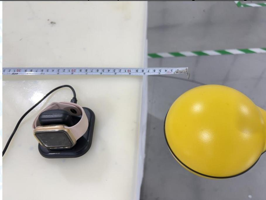
**H-Field Strength- 15 cm****Test Position E - Exposure photo from top surface**
