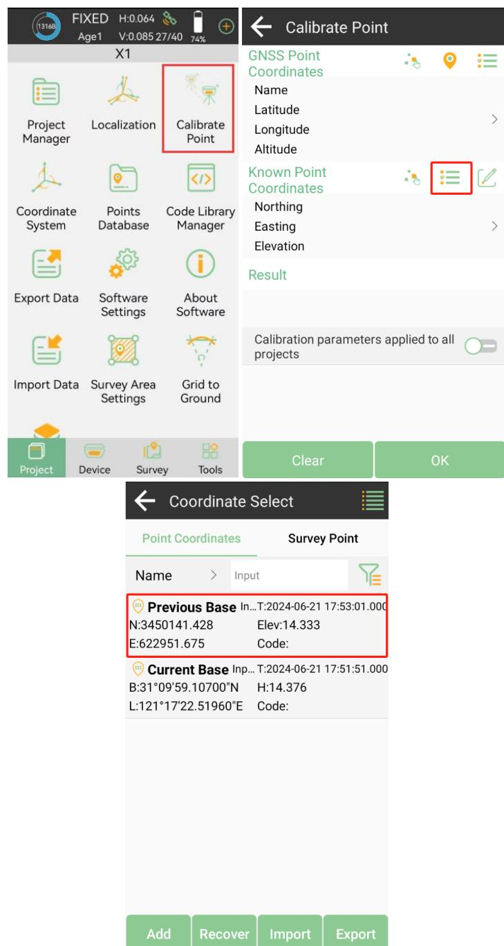
For the GNSS Point Coordinates, you can click the surveying icon to measure under the current base directly.
