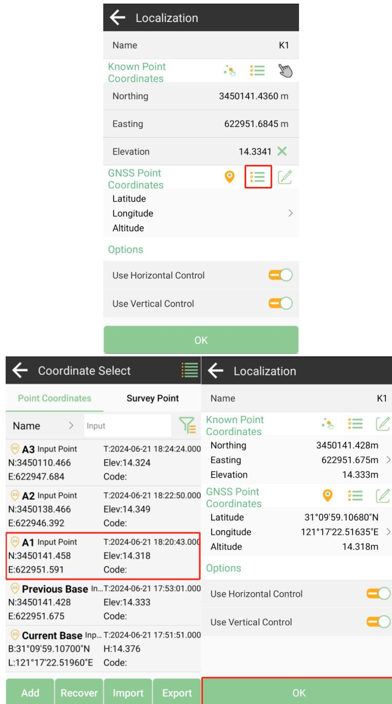
Add the remaining point pairs in sequence. You can also enter the known point in point database in advance and select the input points.
