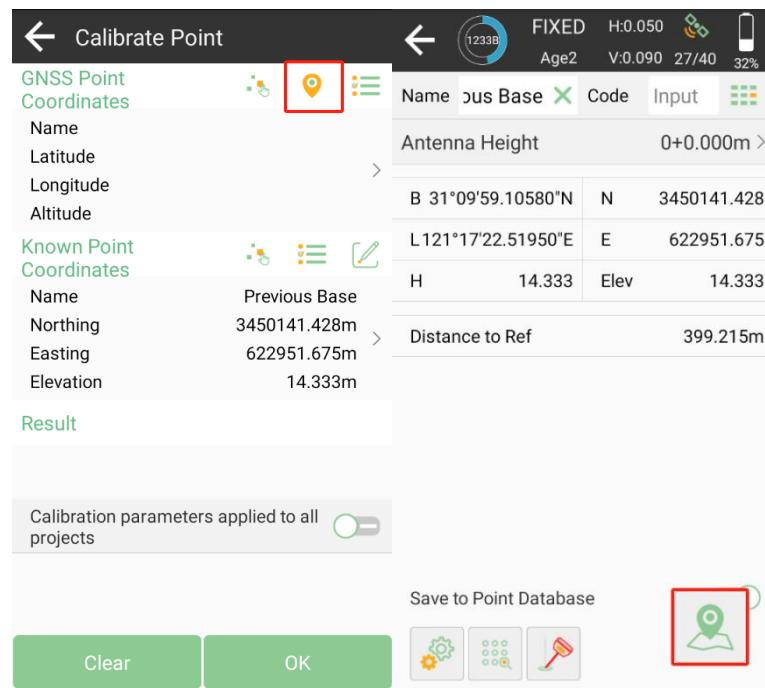
Or measure the GNSS point under the current base station in advance and click to select from the point database.
