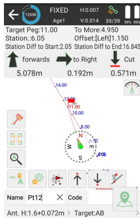
Choose a line to stake, set Offset, Cross-Section Slop and Stakeout by Pile-to-Pile Coordinate parameters.
