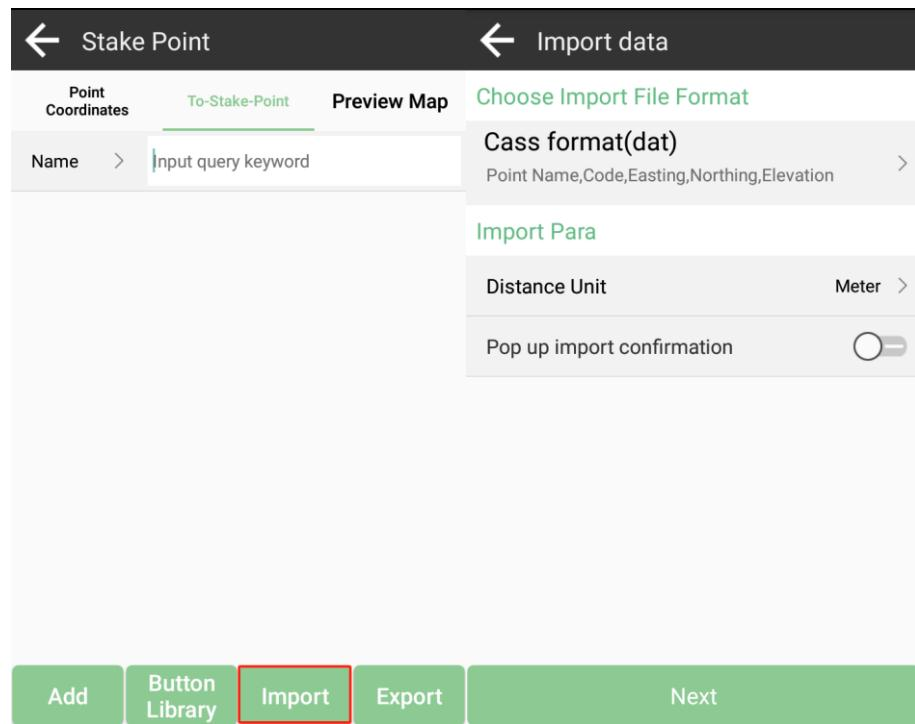
Select a point to stake out, SingularPad provides a navigation map when staking points/lines. The software alerts you when you approach the target point to the set range value.
