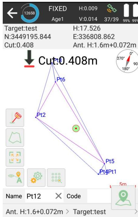
If the current position is not within the design surface, it will prompt “Out of surface!”. If the current position is within the design surface, it will show the fill or excavation value.
