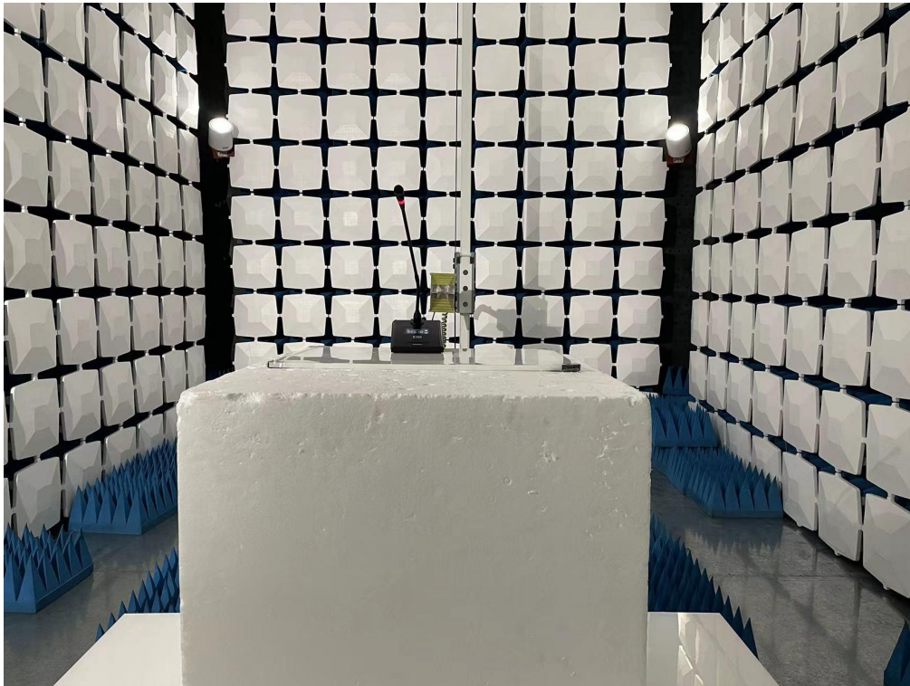
Above 1GHz for radiated emission test setup
