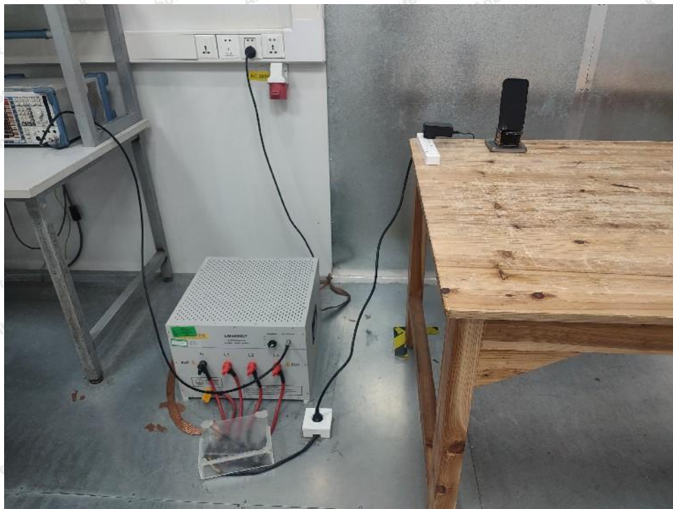
Photo of Conducted Emission Measurement
