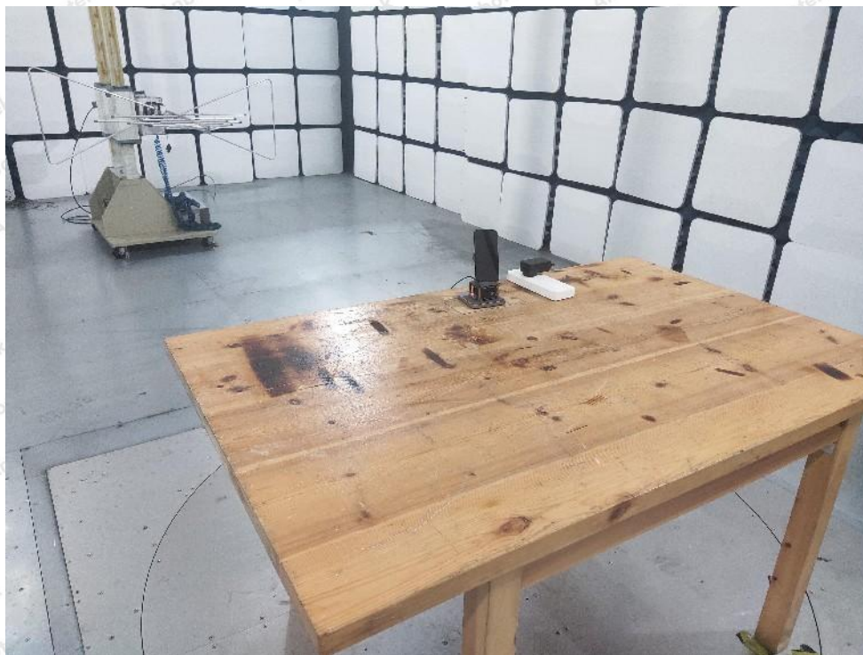
Photo of Radiation Emission Test
