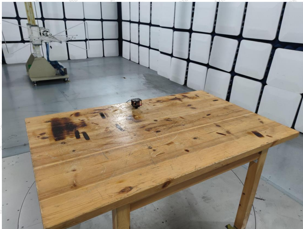
Photo of Radiation Emission Test
