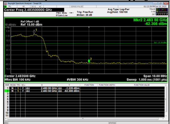
Out Of Band Emission(Right) \pi/4 DQPSK_2-DH5_Channel Hopping
