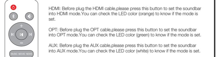
**HDMI:** Before plug the HDMI cable, please press this button to set the soundbar into HDMI mode. You can check the LED color (orange) to know if the mode is set.
