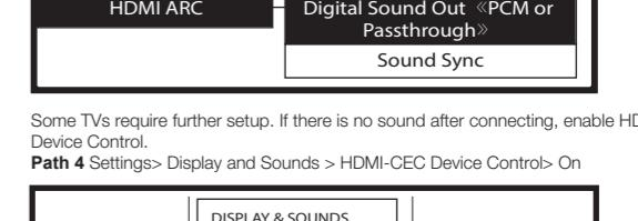
Some TVs require further setup. If there is no sound after connecting, enable HDMI-CEC
