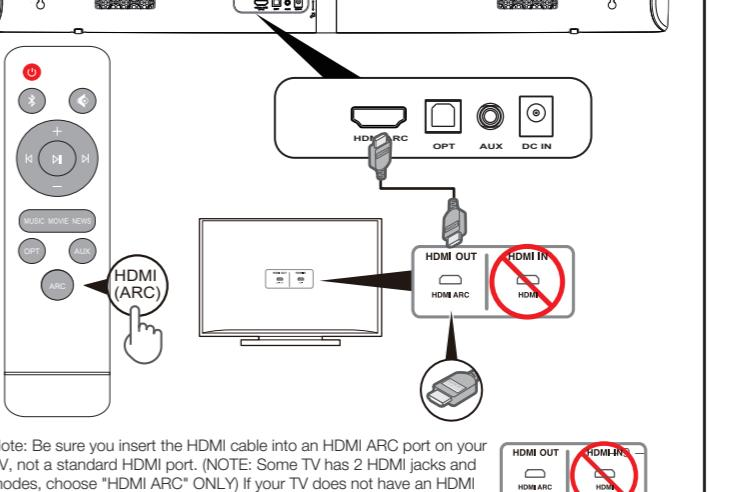
Note: Be sure you insert the HDMI cable into an HDMI ARC port on your TV, not a standard HDMI port. NOT HDMI (ARC) port. NOT HDMI (ARC) port.
