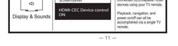
Notes: Allow your TV to control connected CEC-capable HDMI devices using your TV's remote.
