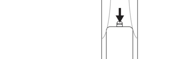
2. Insert the two AAA 1.5V batteries. Match the H and Z symbols on the batteries with the + and - markings inside the compartment.
