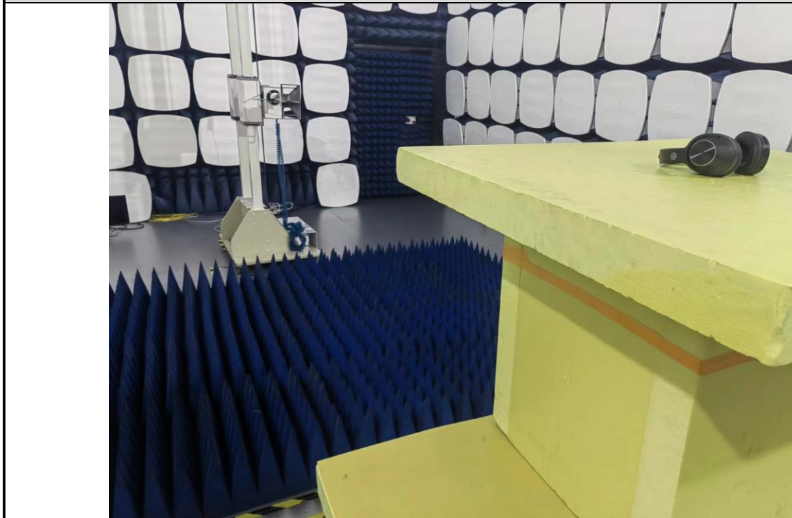
Radiated emission Test Setup (Above 1 GHz)
