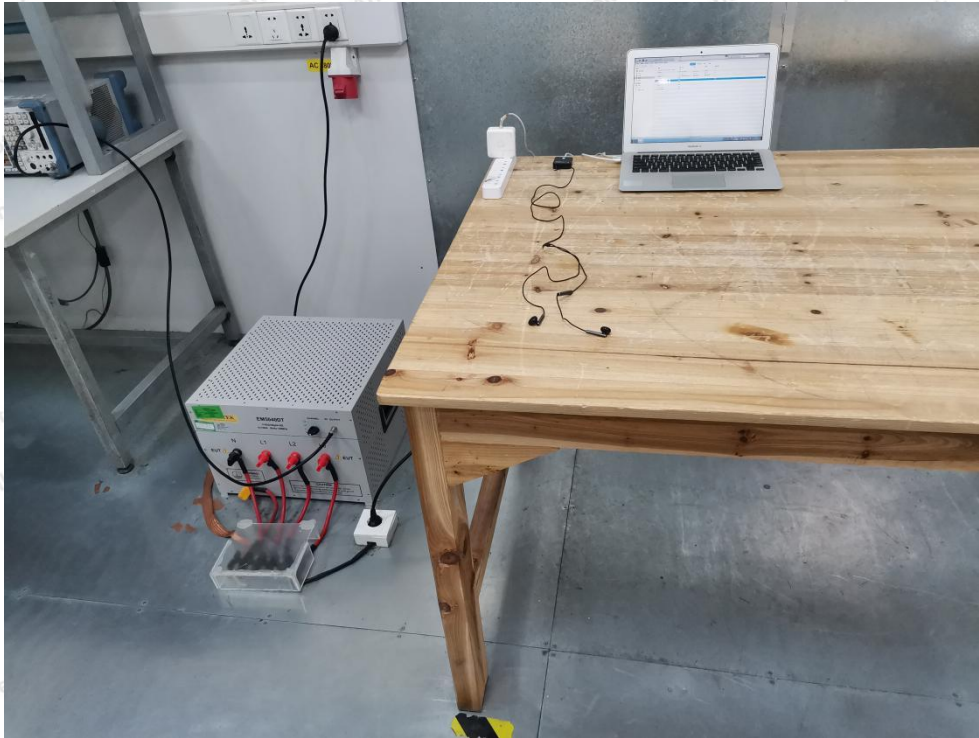
Photo of Conducted Emission Measurement
