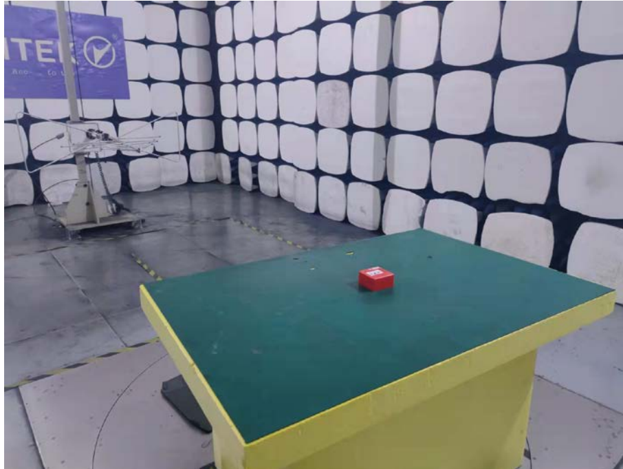
Spurious Emission Test Setup (Above 1GHz)
