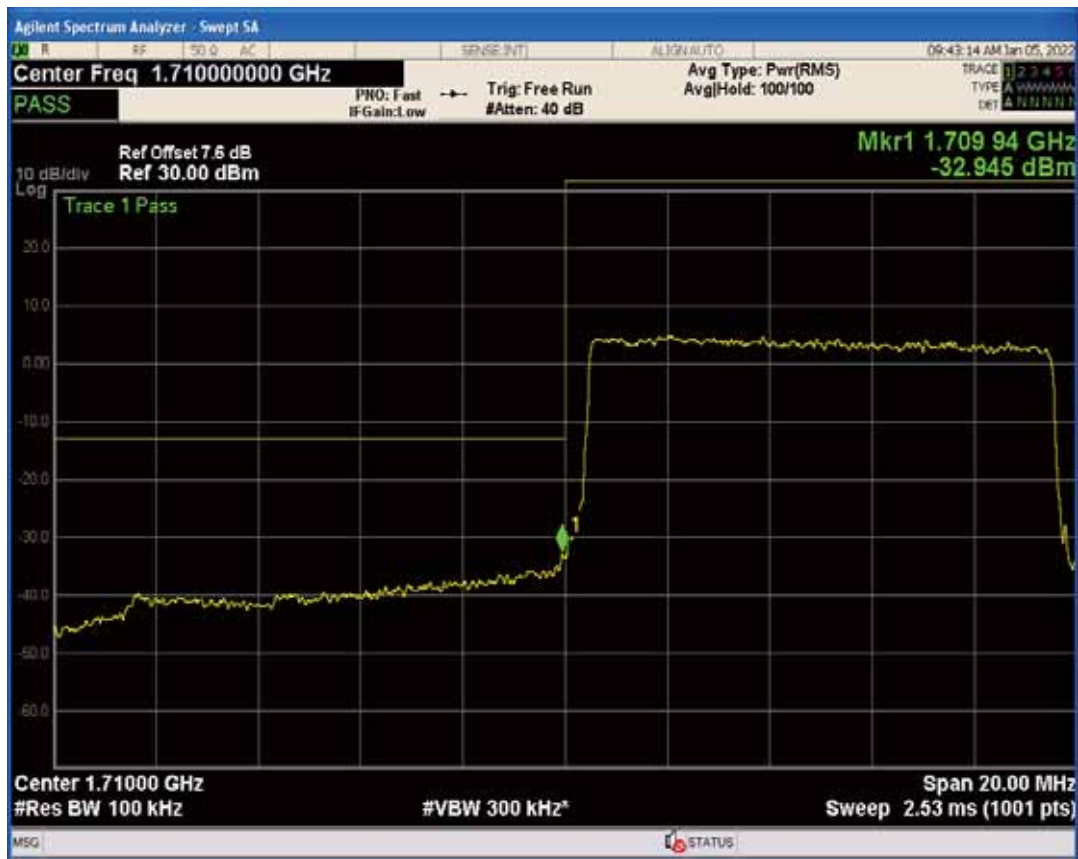
Band4 QPSK BW=10MHz Channel=20000 RB Size=1 Position=#Max
