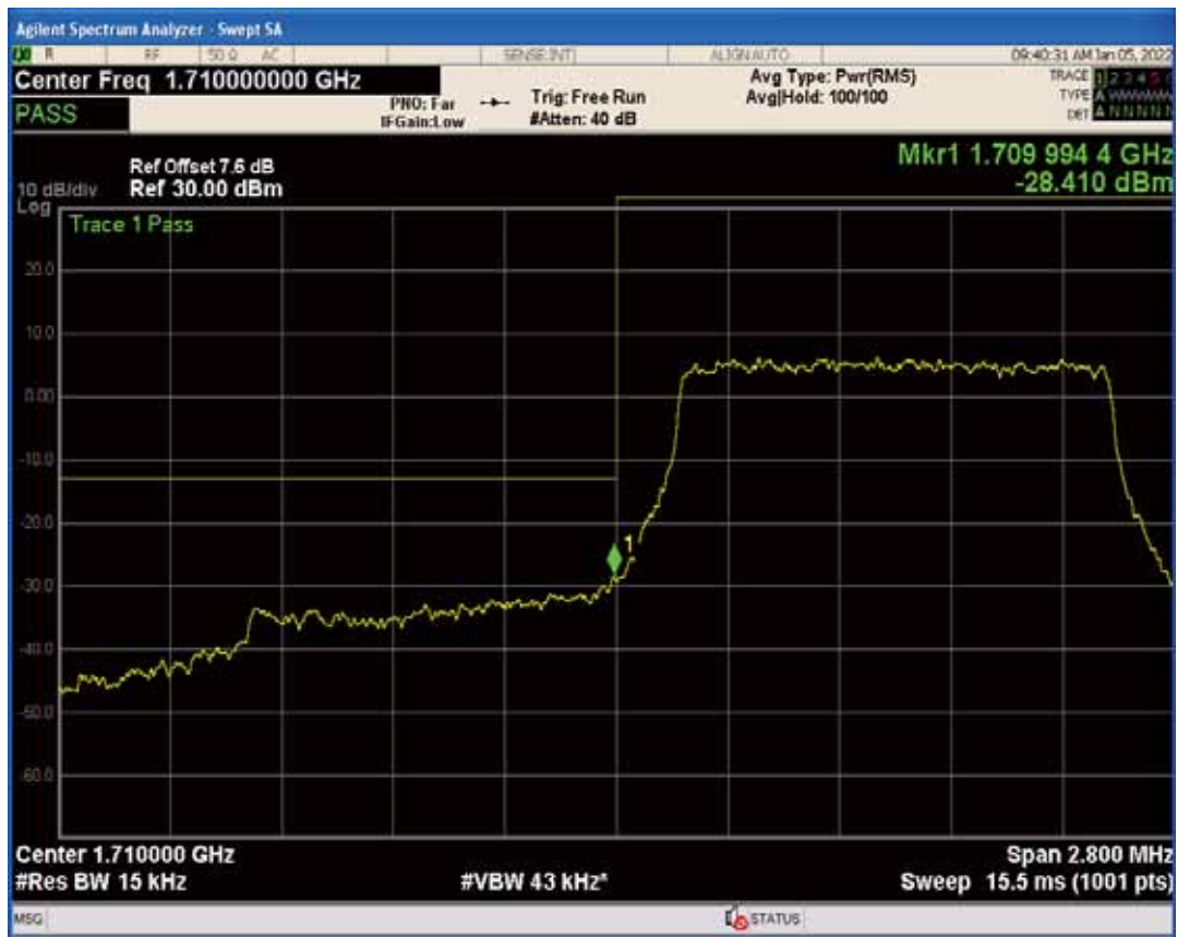
Band4 QAM16 BW=1.4MHz Channel=19957 RB Size=6 Position=#0
