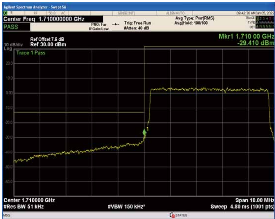
Band4 QPSK BW=5MHz Channel=20375 RB Size=1 Position=#Max
