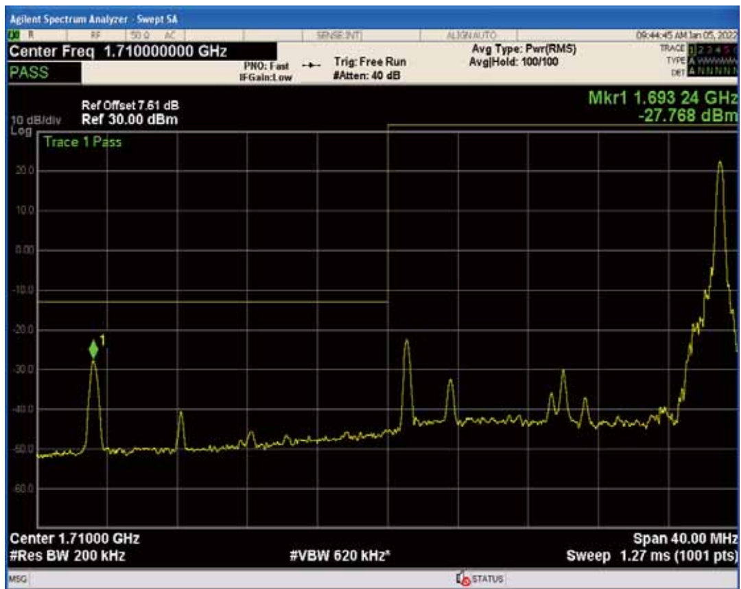
Band4 QAM16 BW=20MHz Channel=20050 RB Size=1 Position=#0
