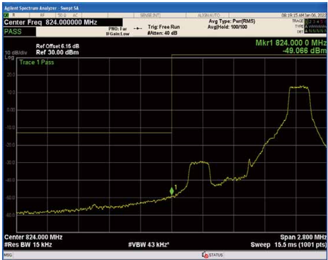
Band26b QPSK BW=1.4MHz Channel=26797 RB Size=6 Position=#0
