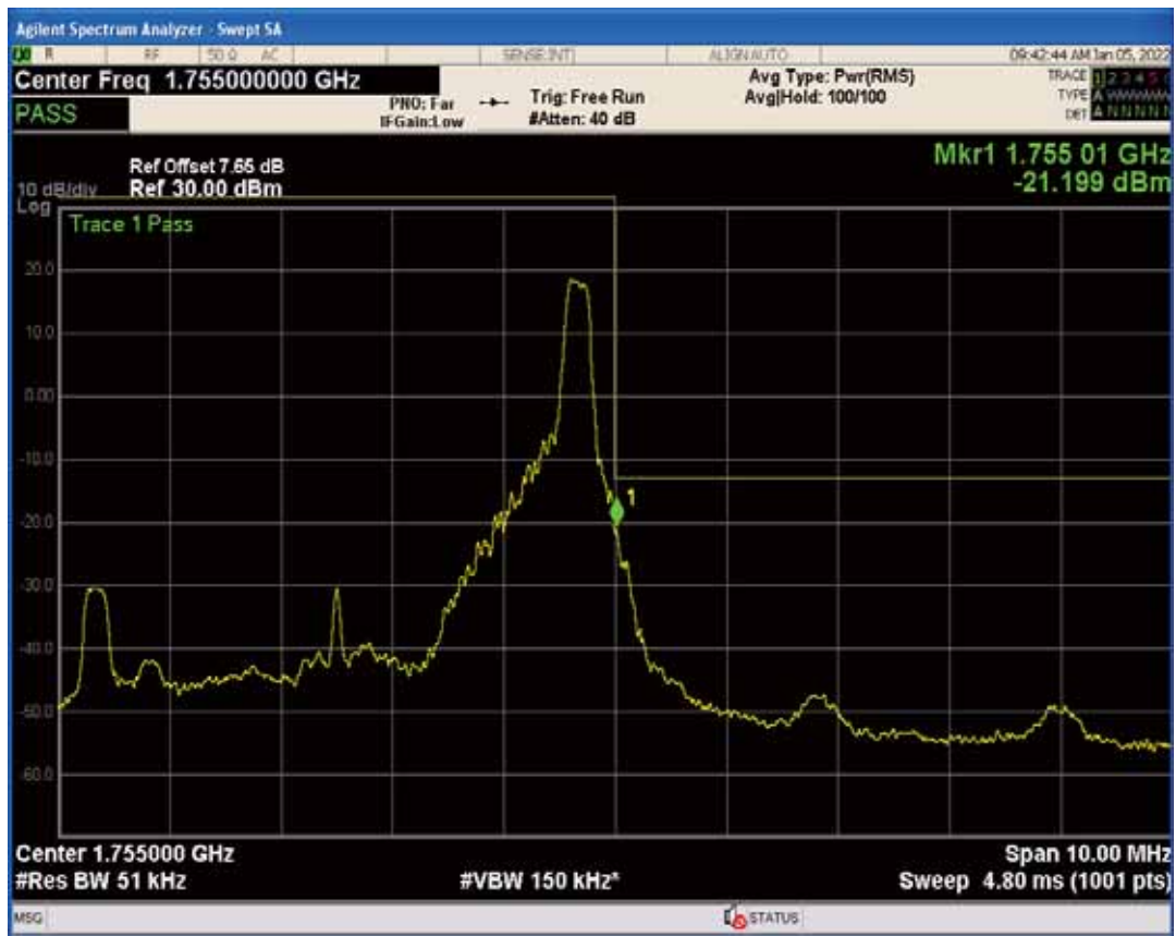
Band4 QPSK BW=5MHz Channel=20375 RB Size=25 Position=#0
