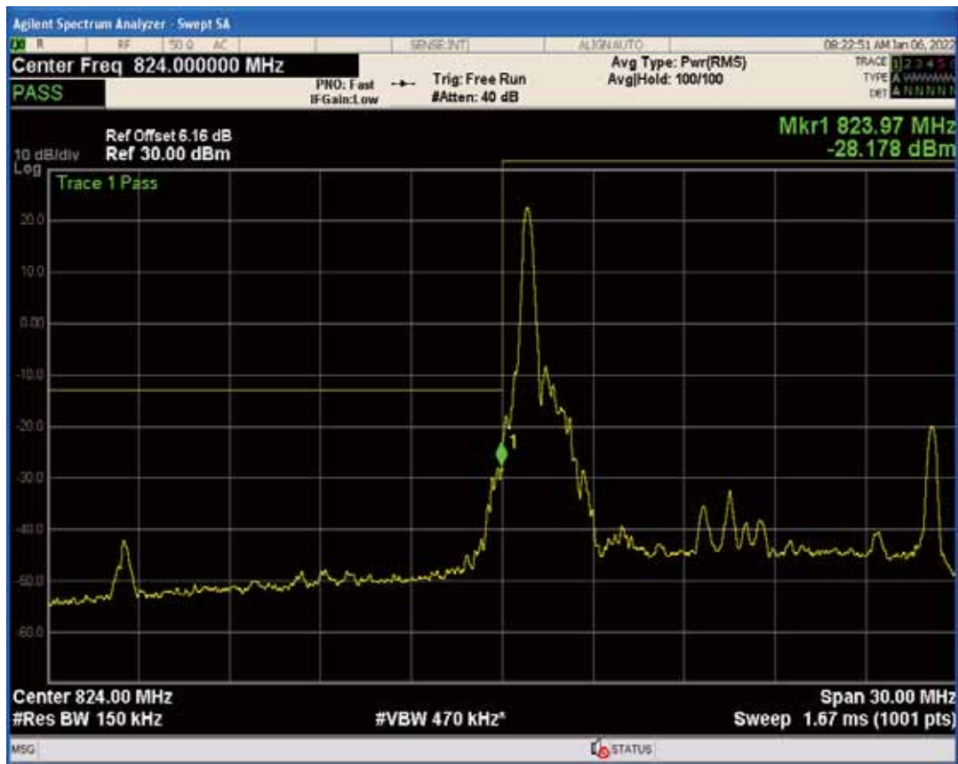
Band26b QPSK BW=15MHz Channel=26865 RB Size=75 Position=#0
