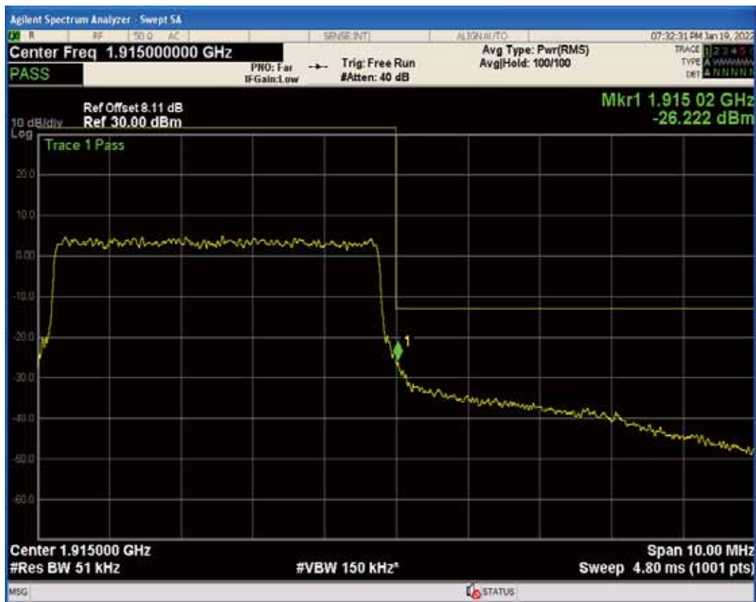
Band25 QPSK BW=5MHz Channel=26665 RB Size=1 Position=#Max
