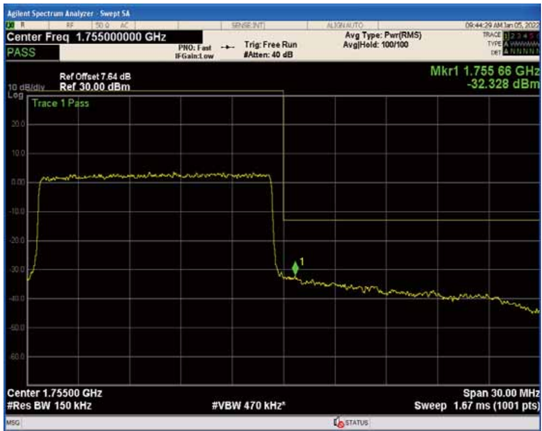
Band4 QPSK BW=20MHz Channel=20050 RB Size=1 Position=#0
