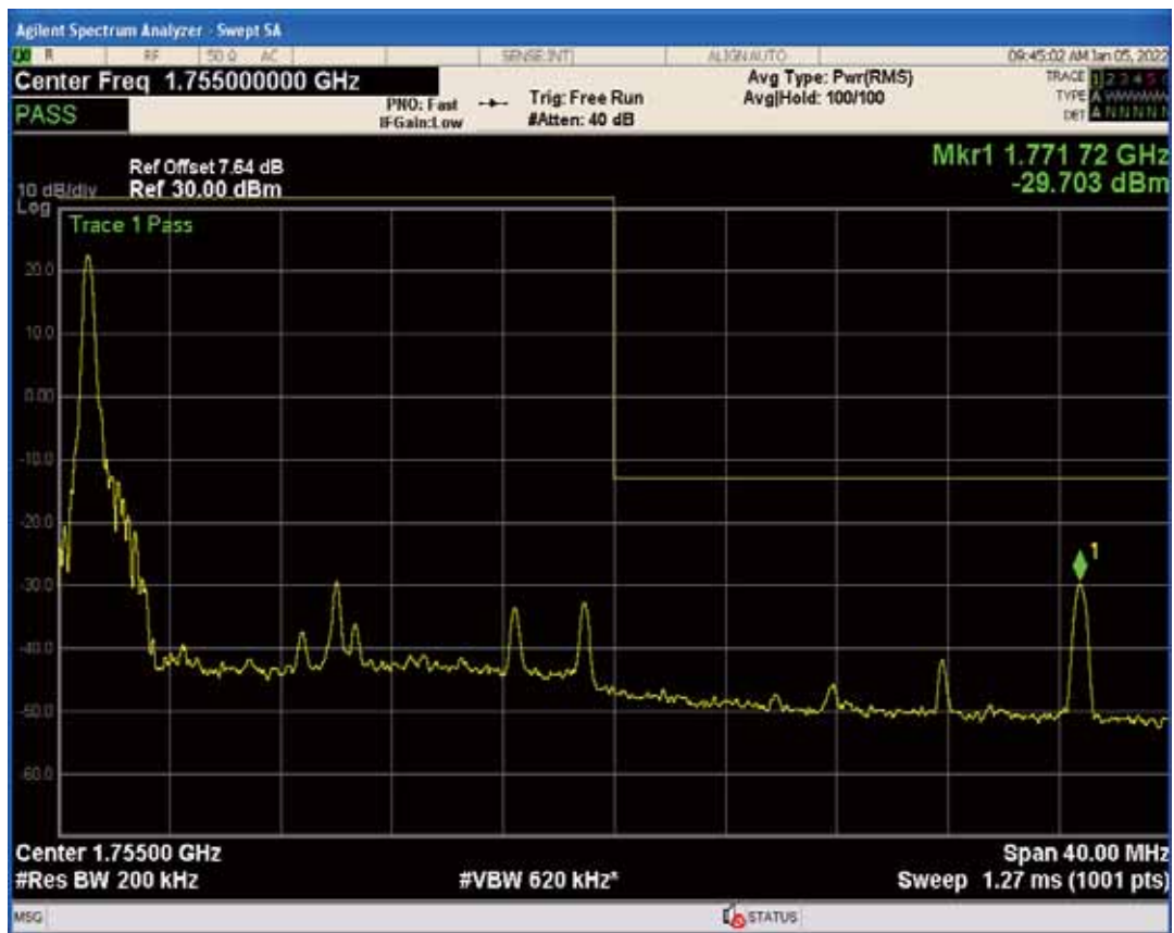
Band4 QPSK BW=20MHz Channel=20300 RB Size=1 Position=#Max
