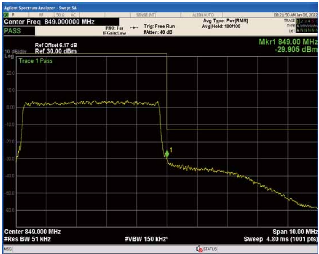
Band26b QPSK BW=10MHz Channel=26840 RB Size=1 Position=#0
