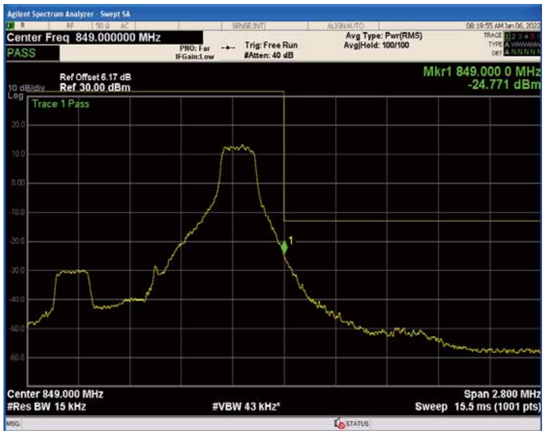
Band26b QAM16 BW=1.4MHz Channel=27033 RB Size=6 Position=#0
