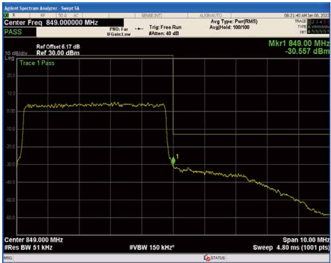
Band26b QAM16 BW=5MHz Channel=27015 RB Size=1 Position=#Max
