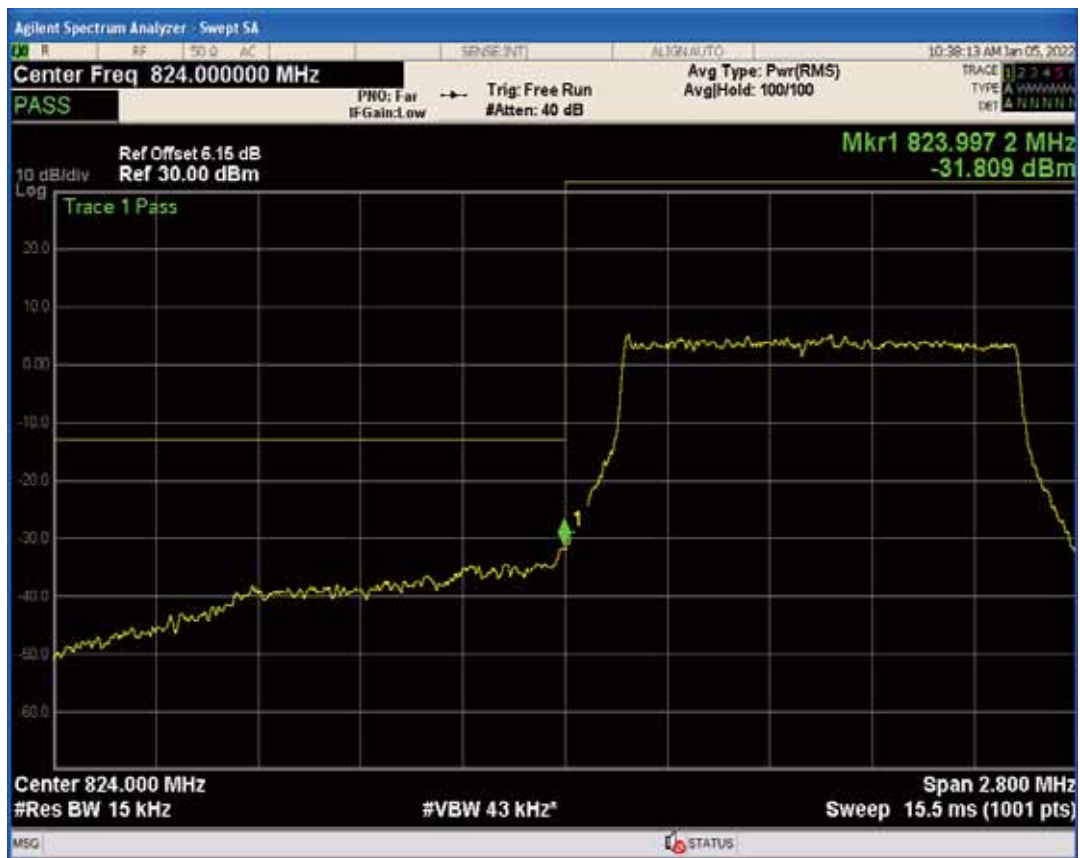
Band5 QPSK BW=1.4MHz Channel=20643 RB Size=1 Position=#Max
