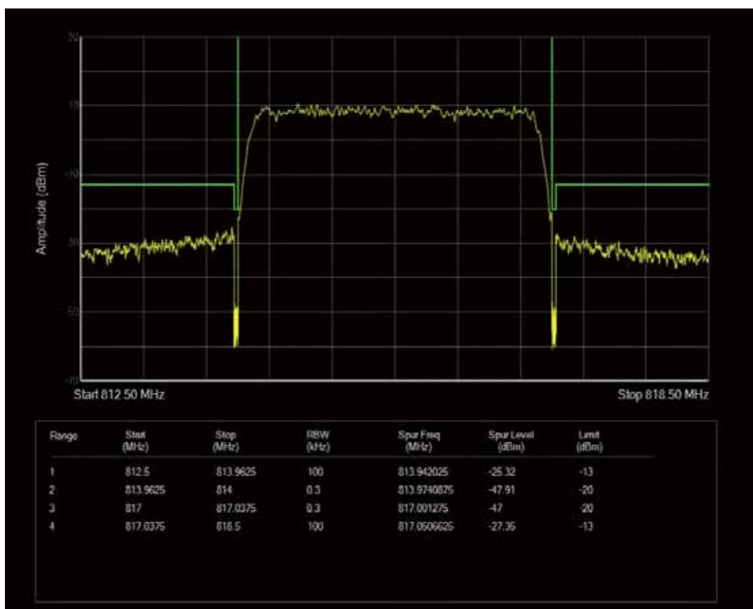
Band26a QAM16 BW=3MHz Channel=26705 RB Size=1 Position=#0
