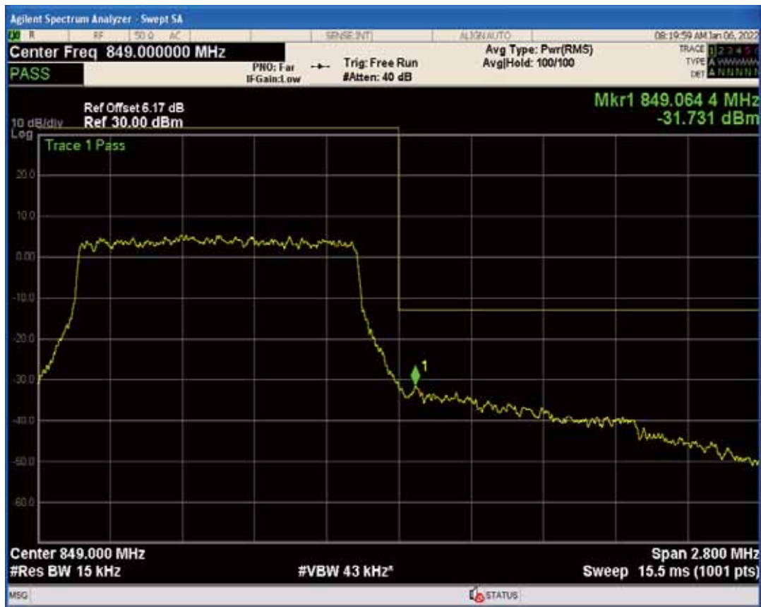
Band26b QPSK BW=3MHz Channel=26805 RB Size=1 Position=#0
