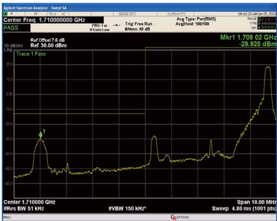
Band4 QAM16 BW=5MHz Channel=19975 RB Size=1 Position=#0
