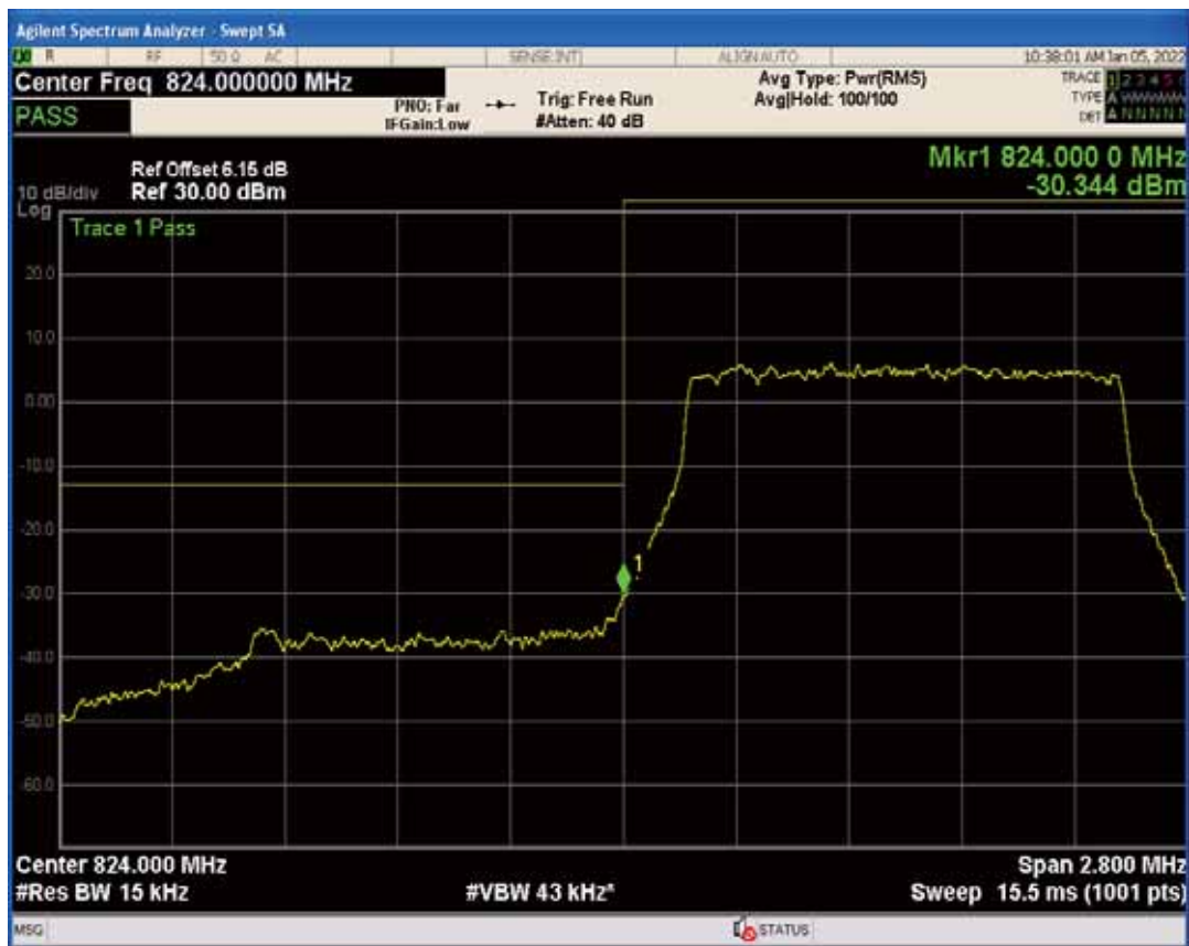
Band5 QAM16 BW=1.4MHz Channel=20407 RB Size=1 Position=#0
