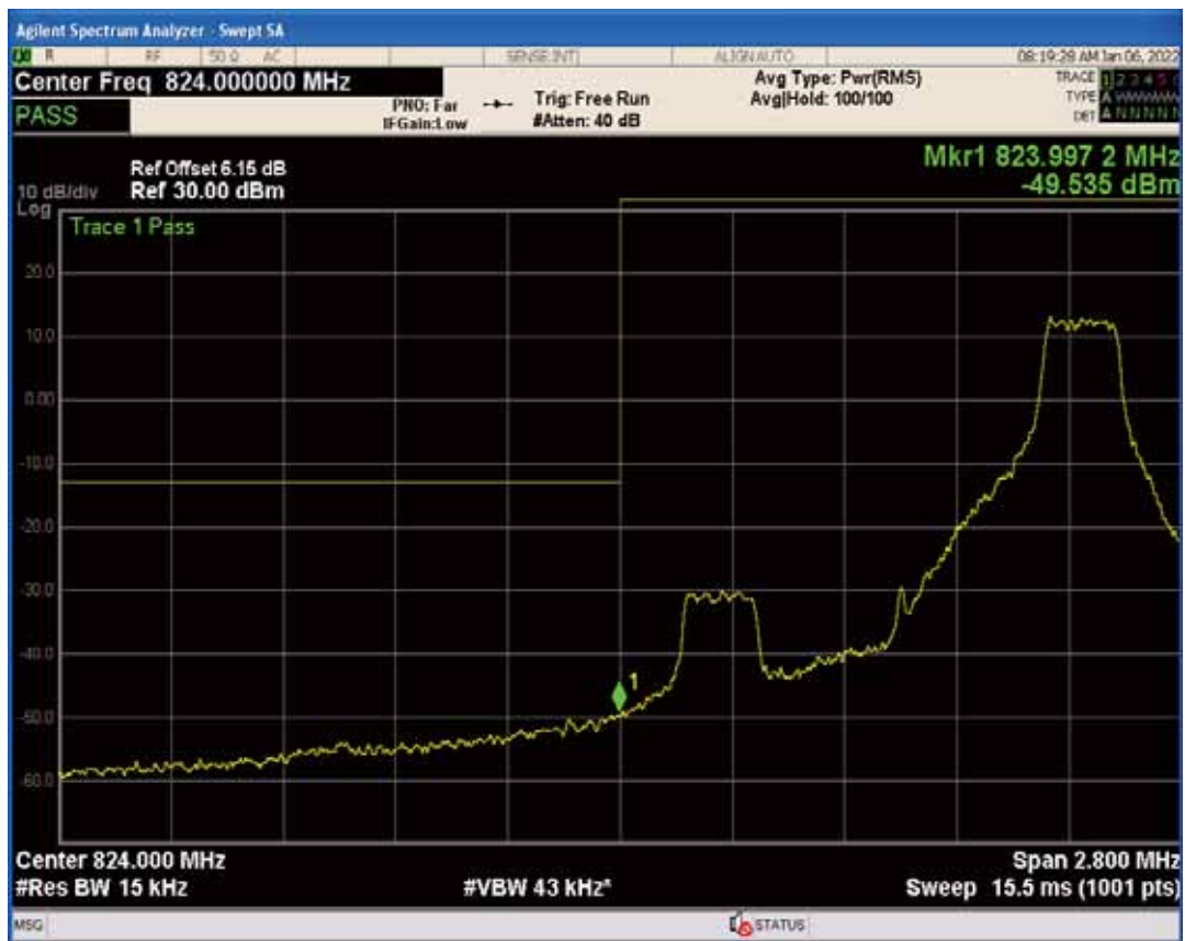
Band26b QAM16 BW=1.4MHz Channel=26797 RB Size=6 Position=#0
