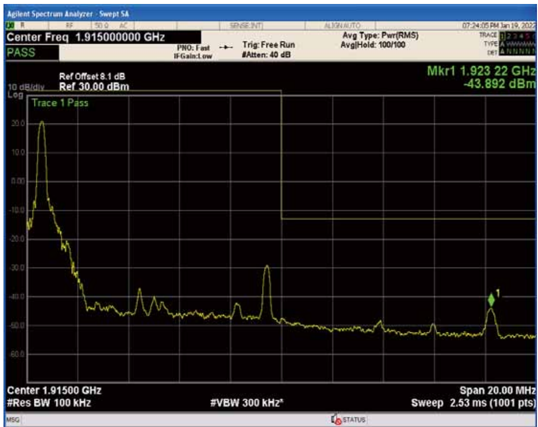
Band25 QPSK BW=15MHz Channel=26115 RB Size=75 Position=#0
