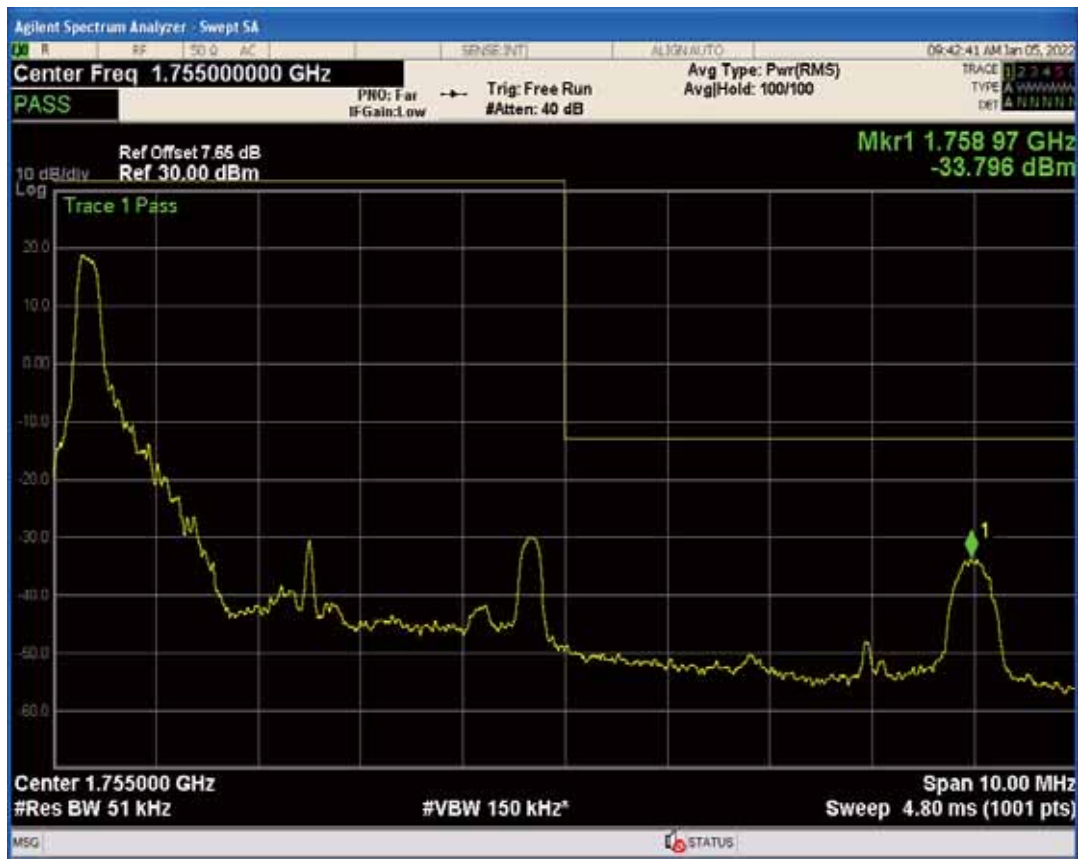
Band4 QAM16 BW=5MHz Channel=19975 RB Size=25 Position=#0
