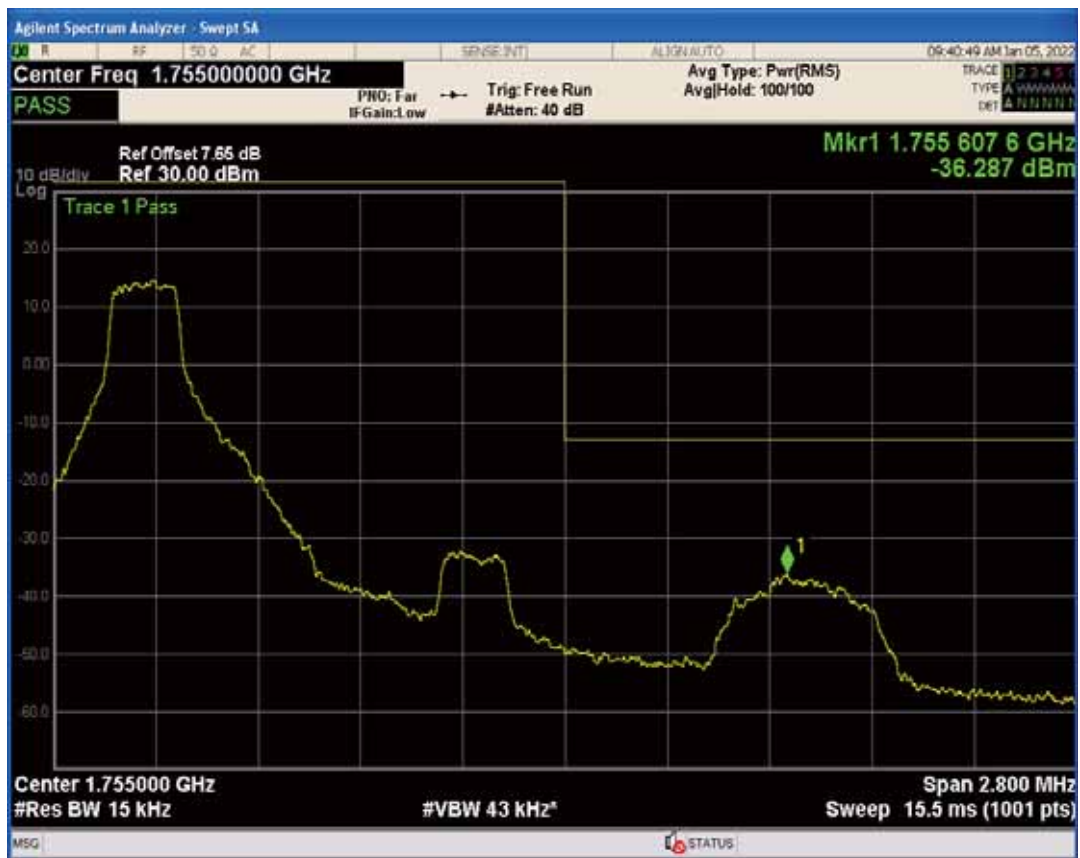
Band4 QPSK BW=1.4MHz Channel=20393 RB Size=1 Position=#Max
