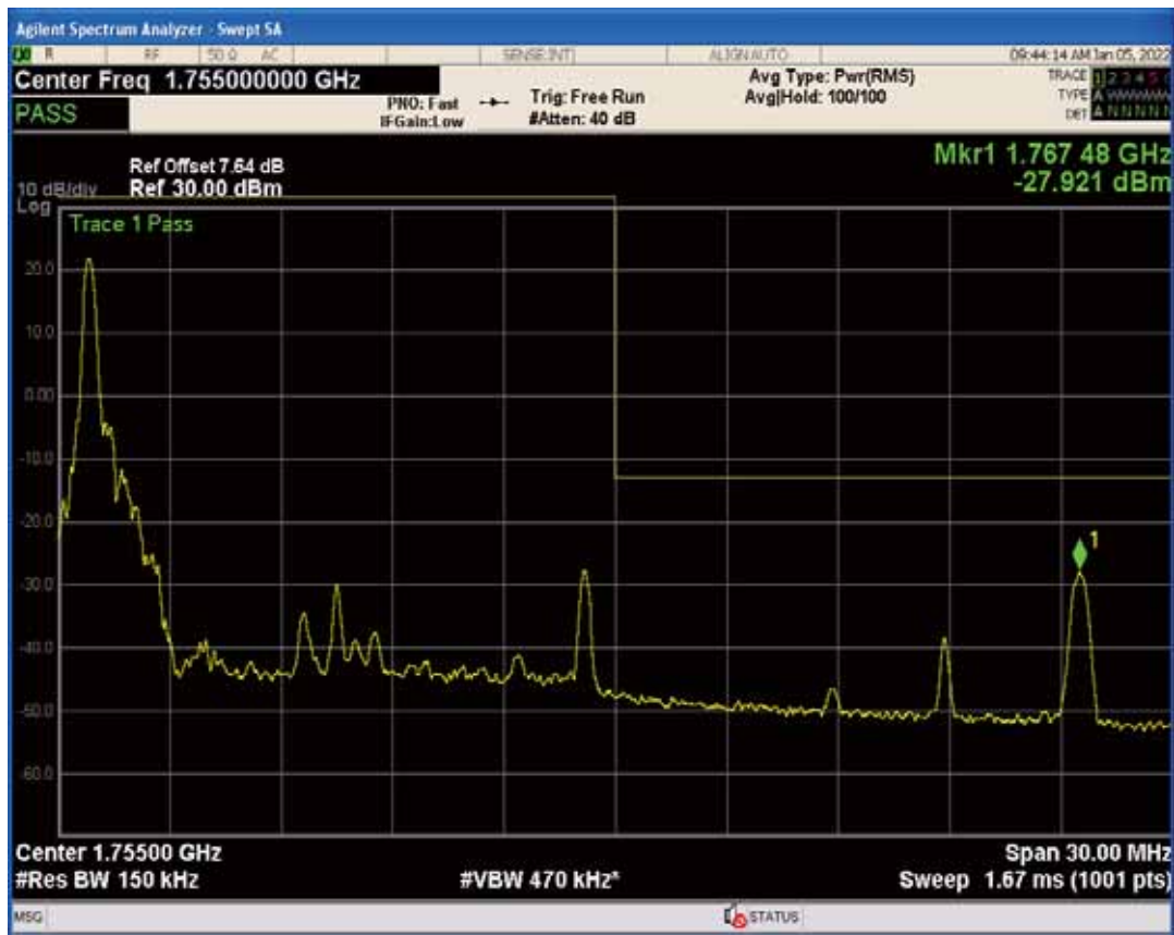
Band4 QAM16 BW=15MHz Channel=20025 RB Size=75 Position=#0
