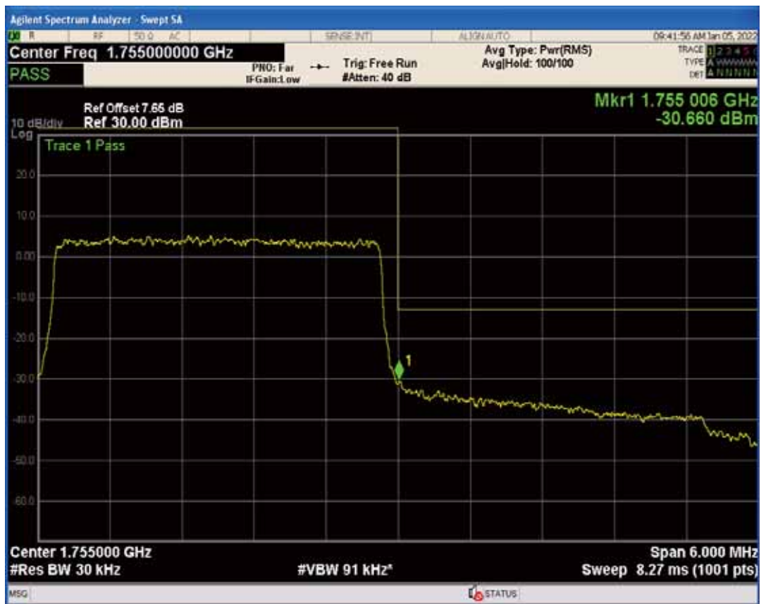
Band4 QAM16 BW=3MHz Channel=20385 RB Size=1 Position=#0
