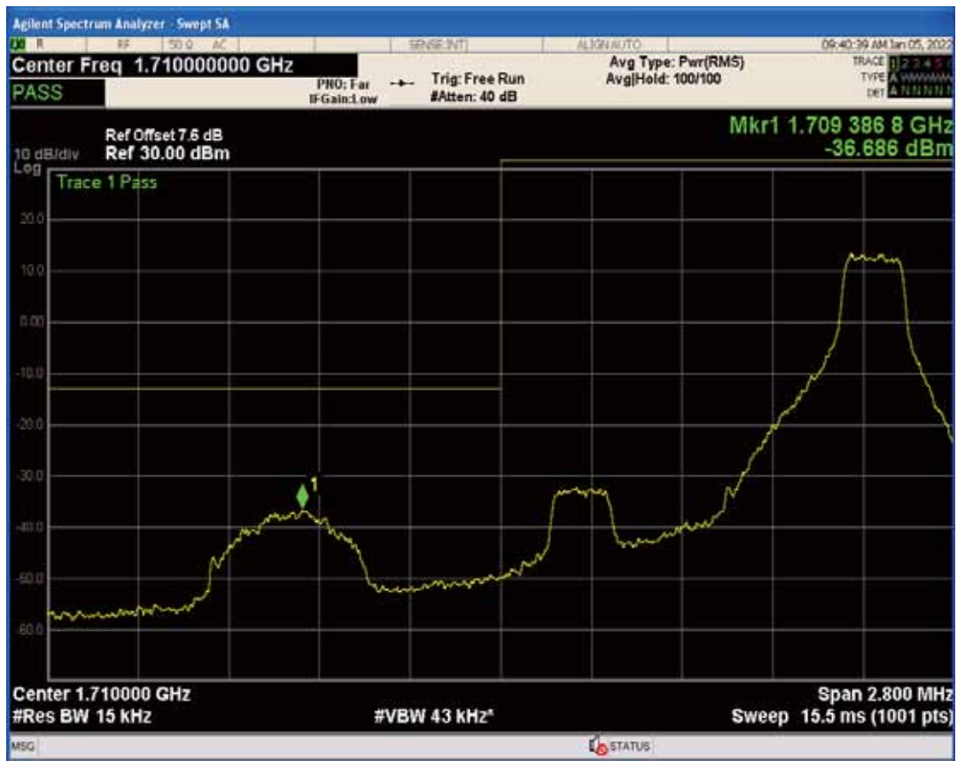
Band4 QPSK BW=1.4MHz Channel=20393 RB Size=1 Position=#0
