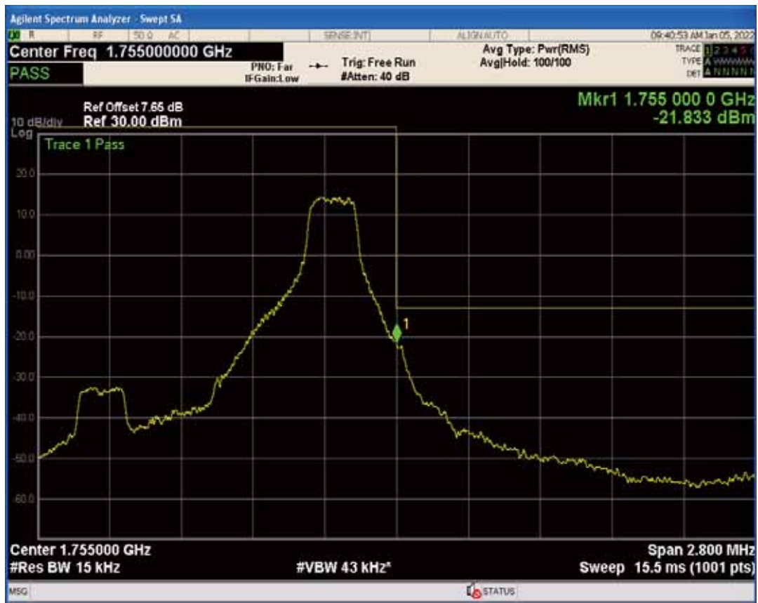
Band4 QPSK BW=1.4MHz Channel=20393 RB Size=6 Position=#0
