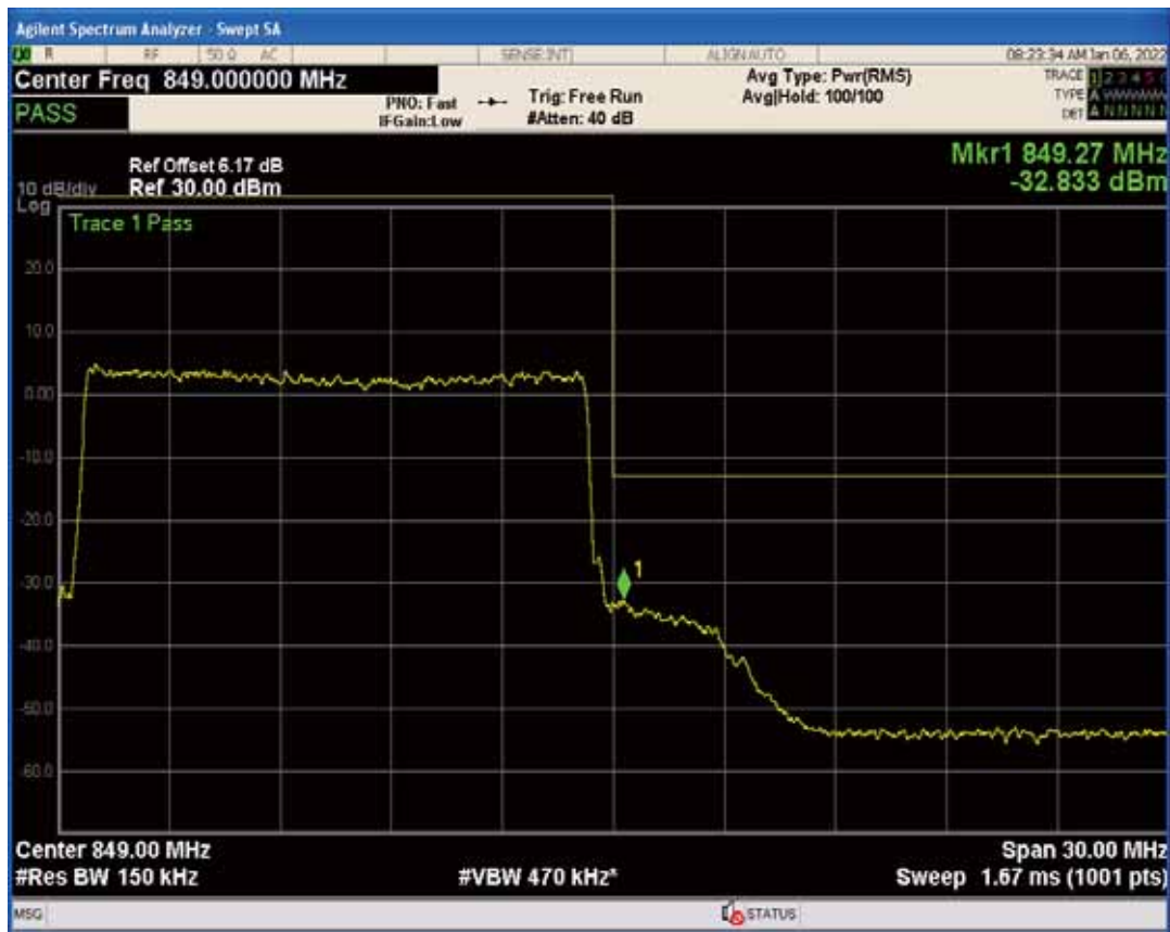
Band4 QPSK BW=1.4MHz Channel=19957 RB Size=1 Position=#0
