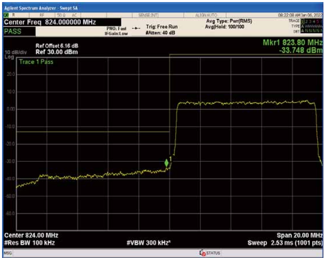
Band26b QPSK BW=10MHz Channel=26840 RB Size=1 Position=#Max
