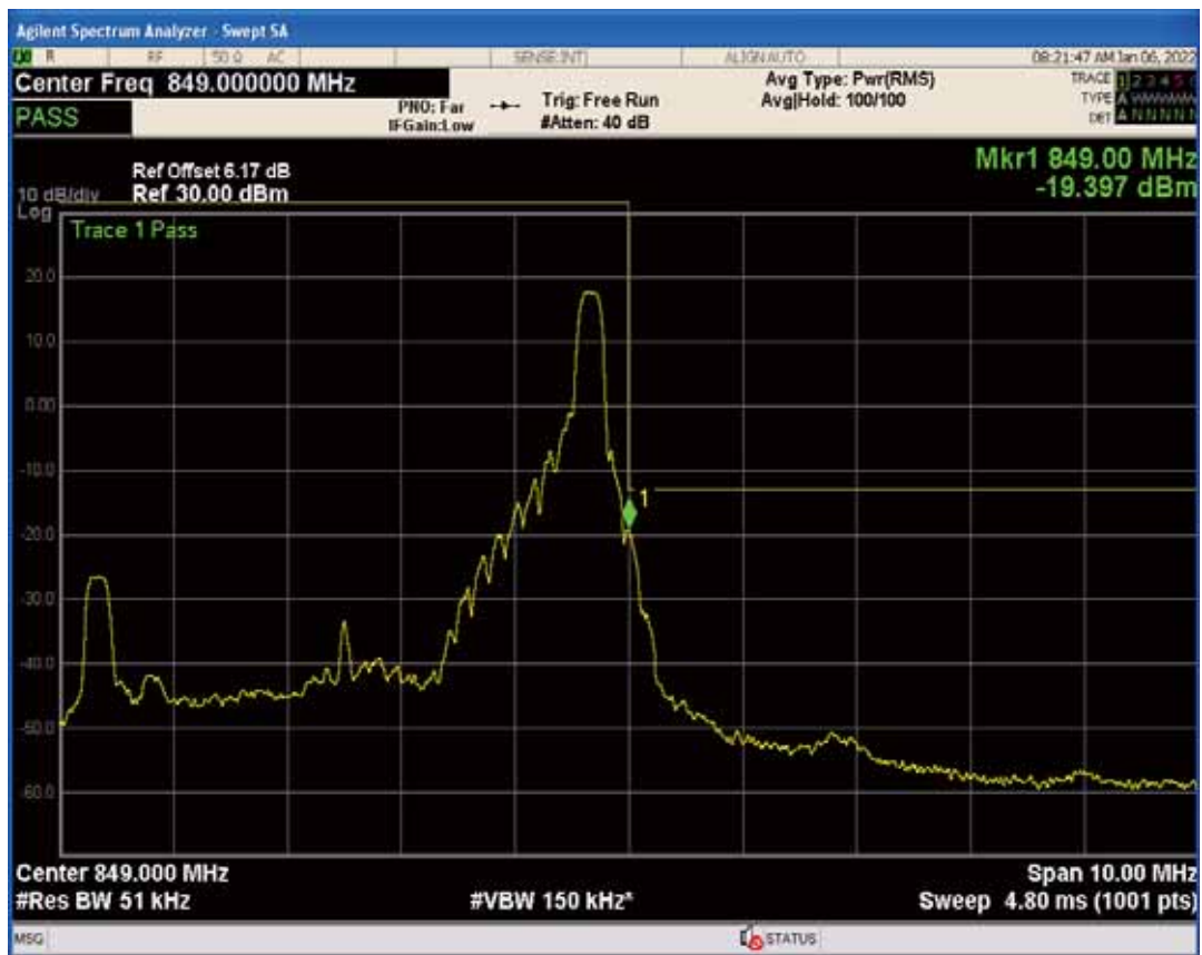
Band26b QAM16 BW=5MHz Channel=27015 RB Size=25 Position=#0
