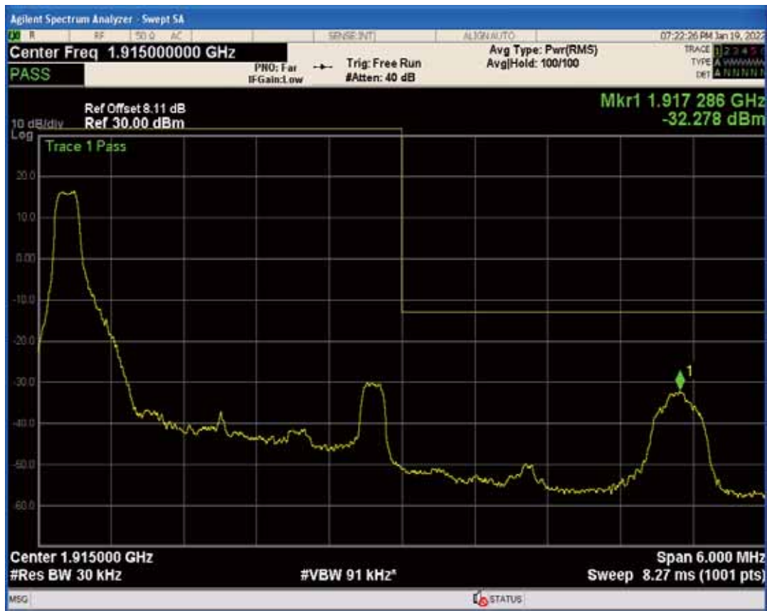
Band25 QPSK BW=3MHz Channel=26675 RB Size=15 Position=#0
