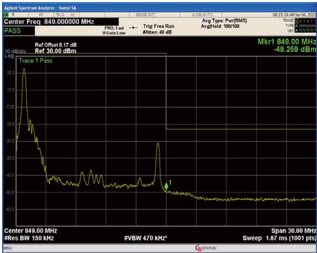
Band26b QPSK BW=15MHz Channel=26965 RB Size=75 Position=#0
