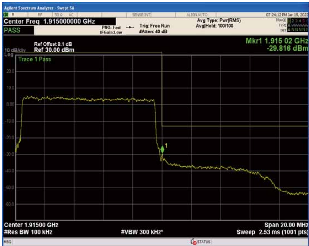
Band25 QPSK BW=10MHz Channel=26090 RB Size=50 Position=#0
