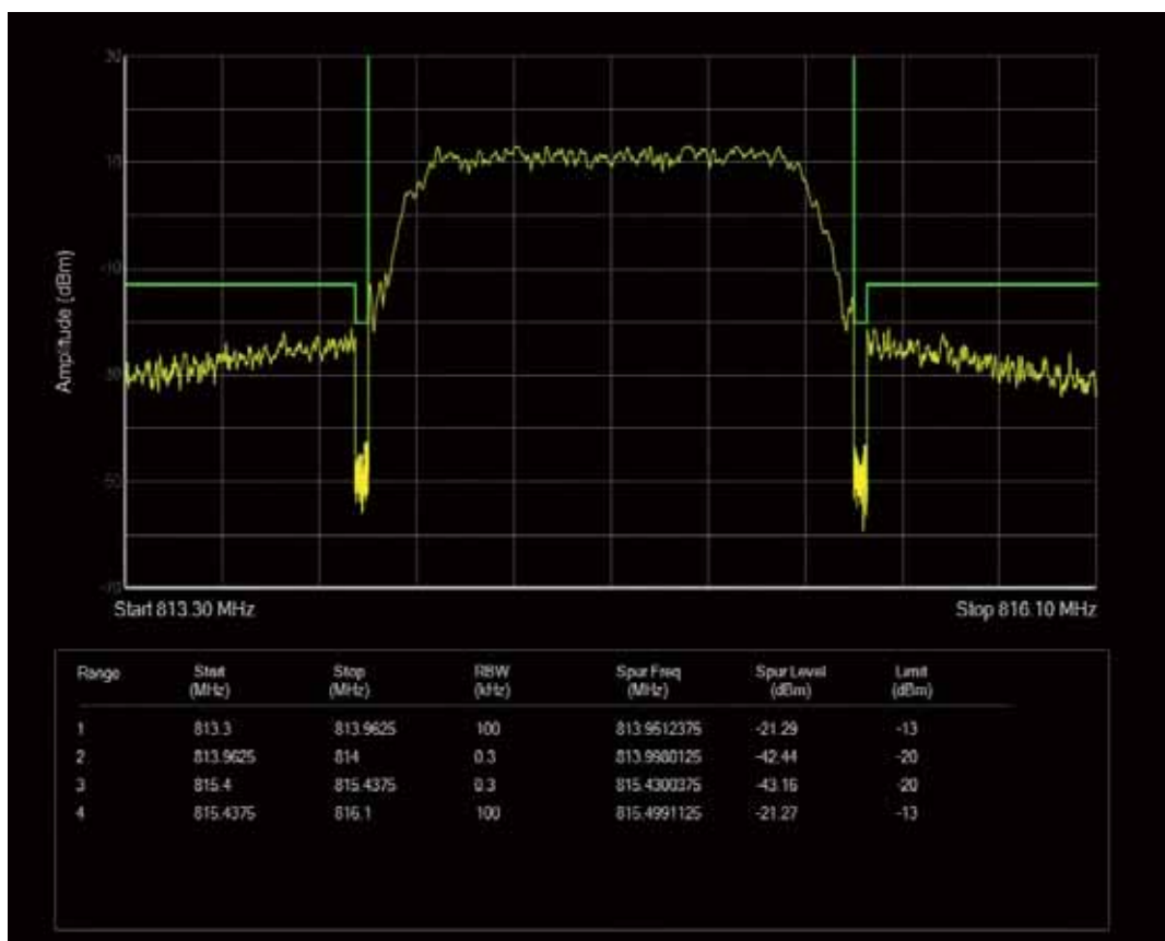
Band26a QPSK BW=1.4MHz Channel=26783 RB Size=1 Position=#0
