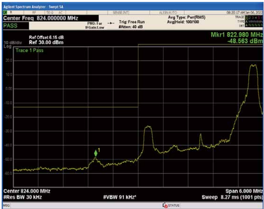
Band26b QAM16 BW=3MHz Channel=26805 RB Size=1 Position=#0
