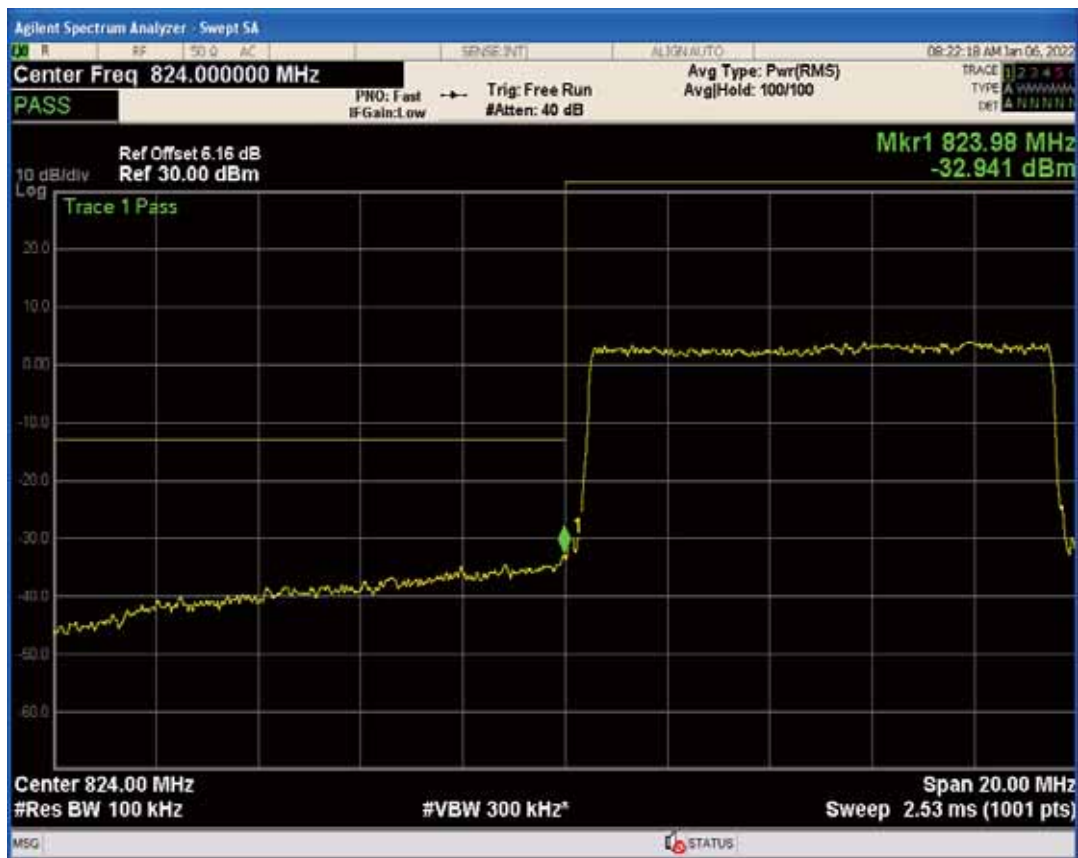
Band26b QAM16 BW=10MHz Channel=26840 RB Size=1 Position=#Max
