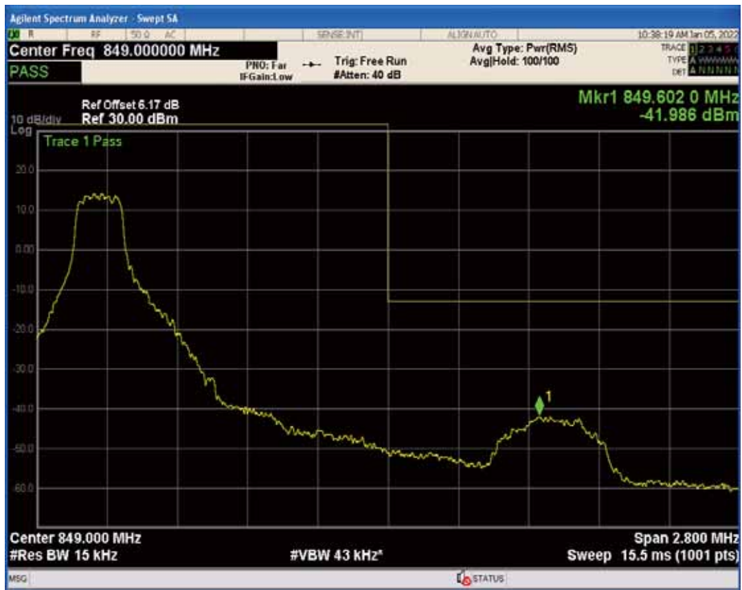
Band5 QAM16 BW=1.4MHz Channel=20407 RB Size=6 Position=#0
