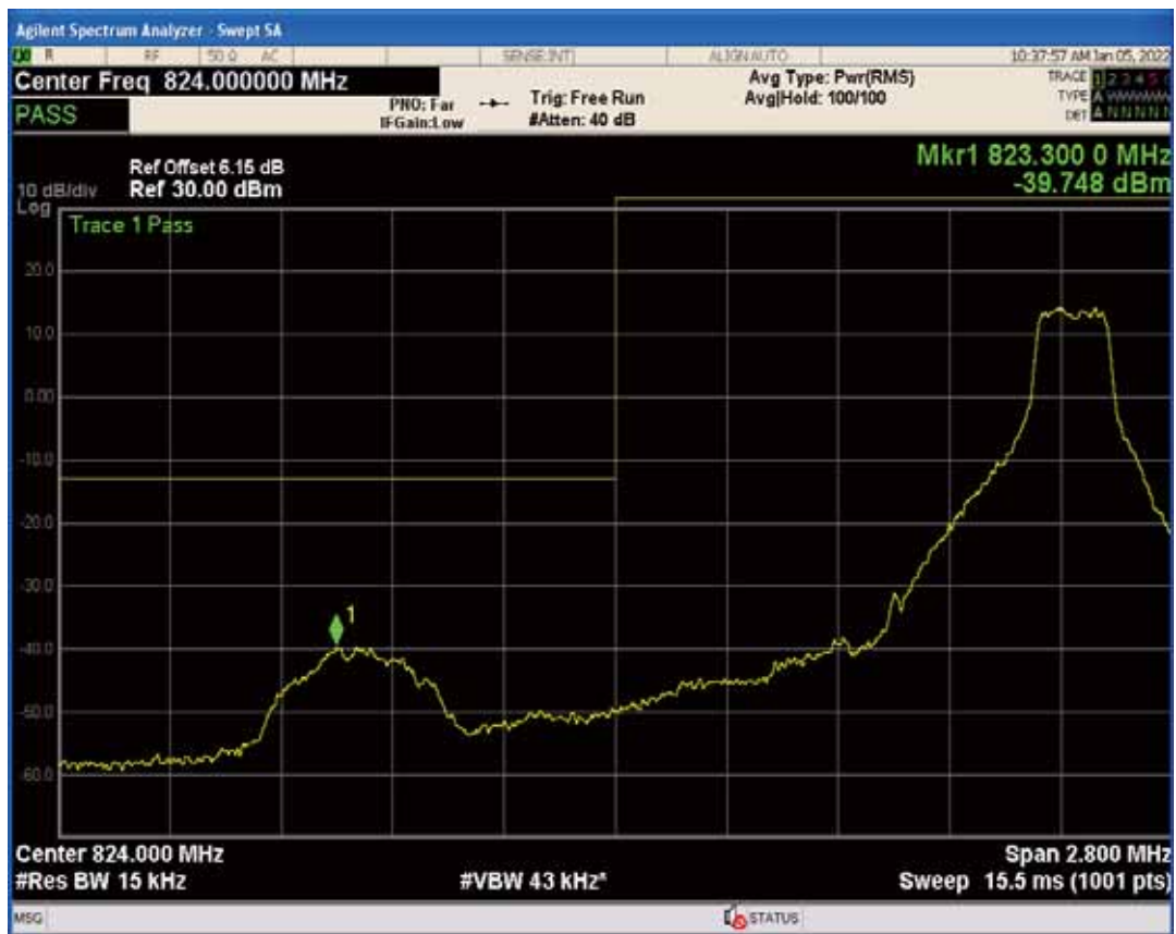
Band5 QPSK BW=1.4MHz Channel=20407 RB Size=1 Position=#0
