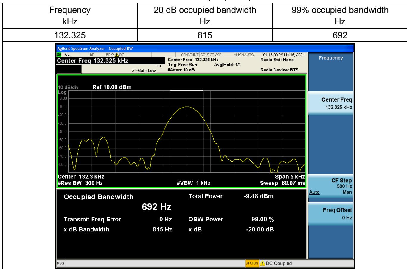
**Note:** Because the measured signal is CW-like, adjusting the RBW per C63.10 would not be practical since measurement bandwidth will always follow the RBW. The RBW is set to 300 Hz to perform the occupied bandwidth test.
