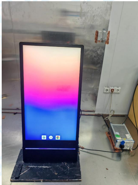
Photo of Setup for Radiated Emission (Below 1 GHz)
