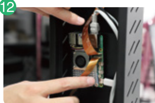
Step12: Connect LAN cables and power cables to the mini boards
