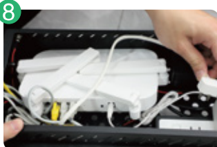
Step8: Plug the power cable to socket
