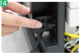
Step14: Fix the bottom ones with M4 thumb screws
