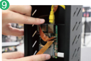
Step9: Connect the other side of LAN cable and power cable to the mini board
