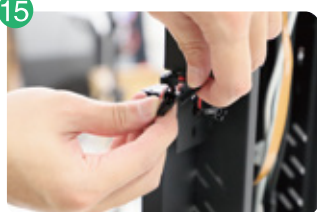
Step15: Connect wires between light bars
