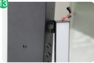
Step13: Attach light bars to the side of bodies
