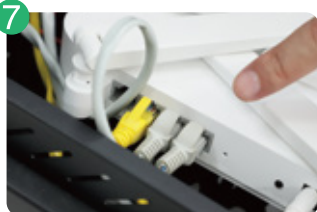
Step7: Connect LAN cables to router
