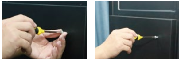
Step 5 : Screw on the for screws for the screen (don't tighten all, just half)
