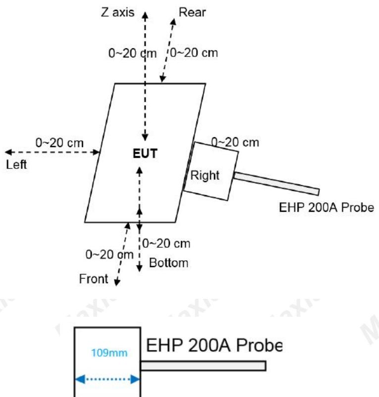
Notes: The EHP 200A Probe has a diameter of 10.9cm and a radius of 5.45cm
