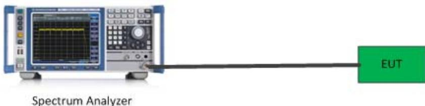
A short RF cable with low cable loss connected to the EUT antenna port. The insert loss of this RF cable/attenuator was offset into the setting of test equipment.
