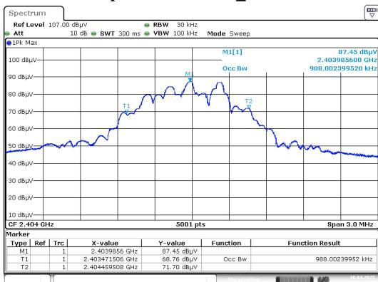
**99% Occupied Bandwidth\_ Middle Channel**
