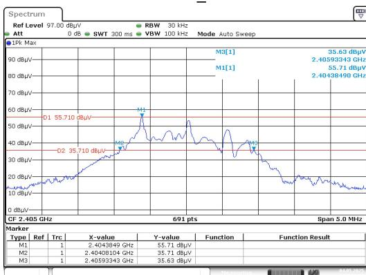
**20 dB Bandwidth \_ Middle Channel**
