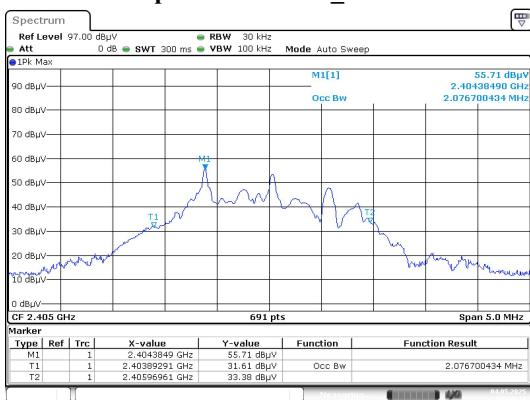
**99% Occupied Bandwidth\_ Middle Channel**
