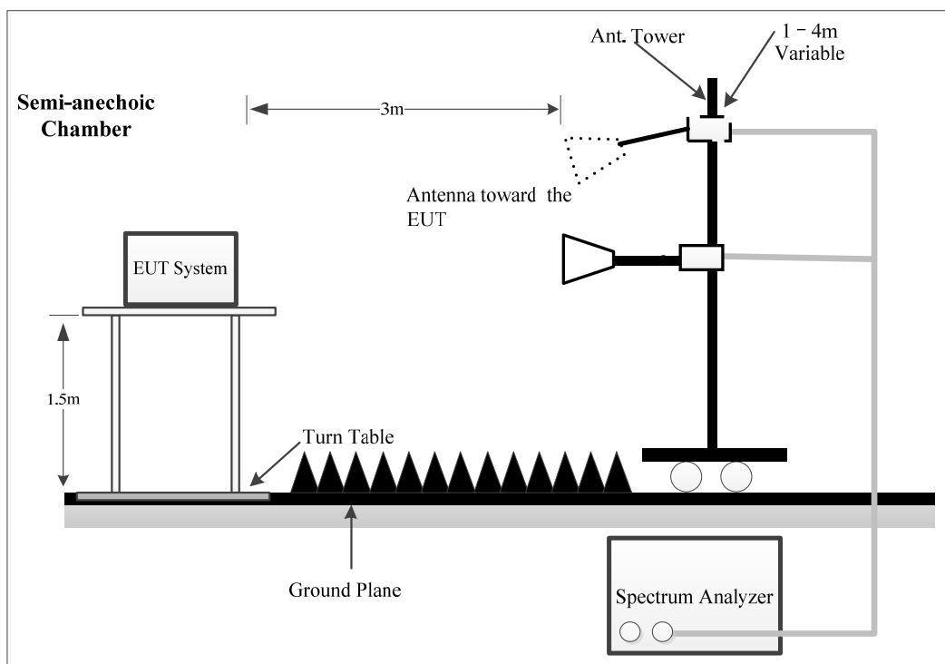
For 9kHz-30MHz test, the lowest height of the magnetic antenna shall be 1 m above the ground and three antenna orientations (parallel, perpendicular, and ground-parallel) shall be measured.
