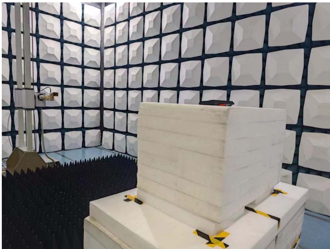
Radiated Emission 18-25GHz View
