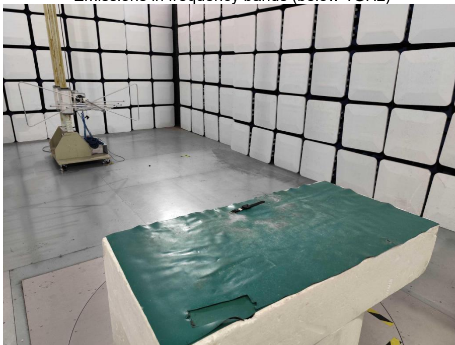
Emissions in frequency bands (below 1GHz)
