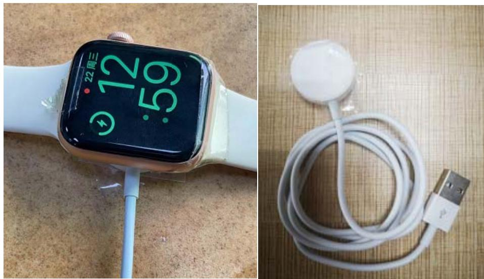
Input voltage/current: DC5V/1.0A
