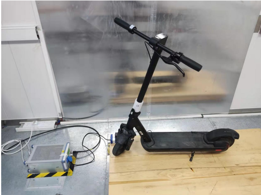
Conducted emission test setup
