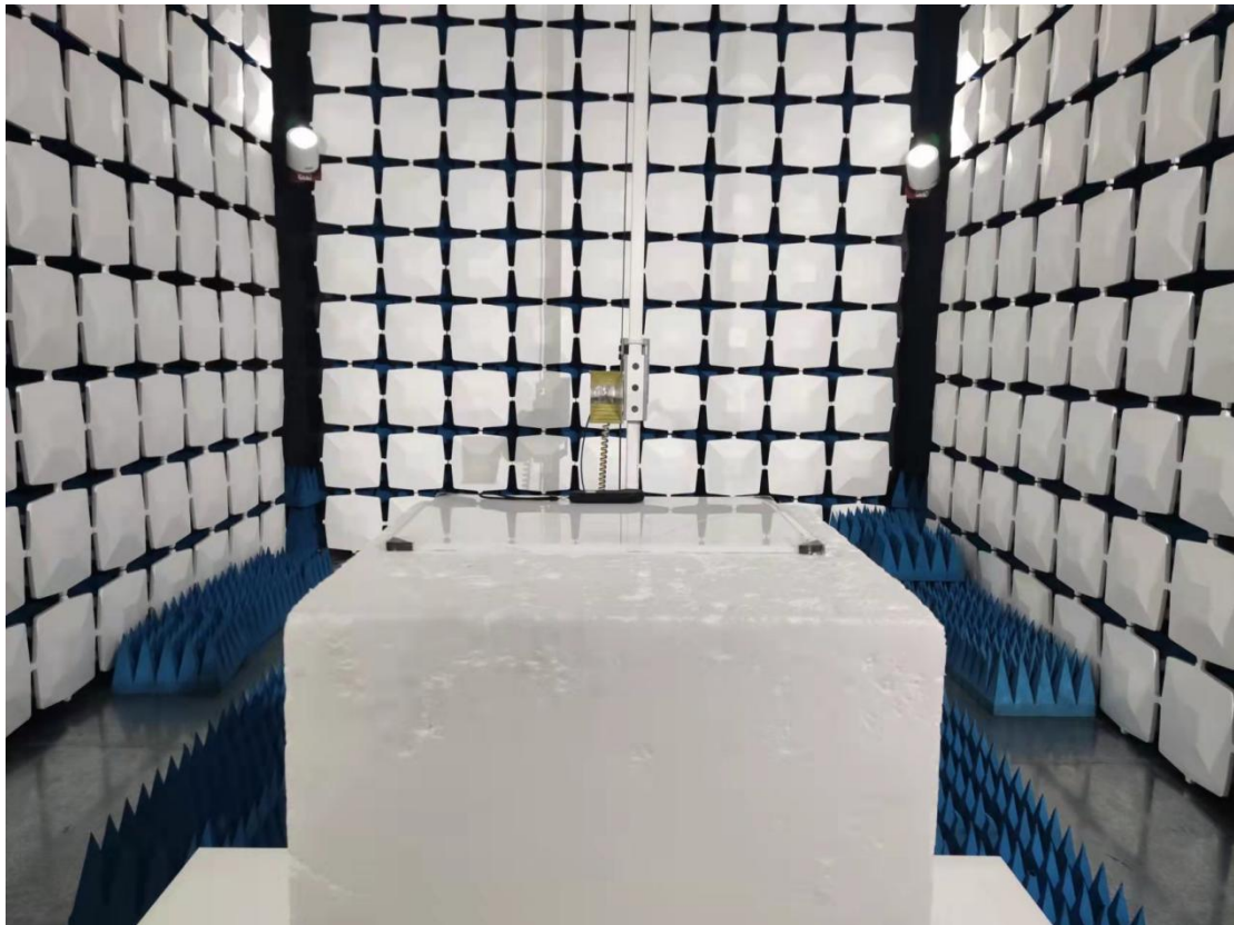
Above 1GHz for radiated emission test setup
