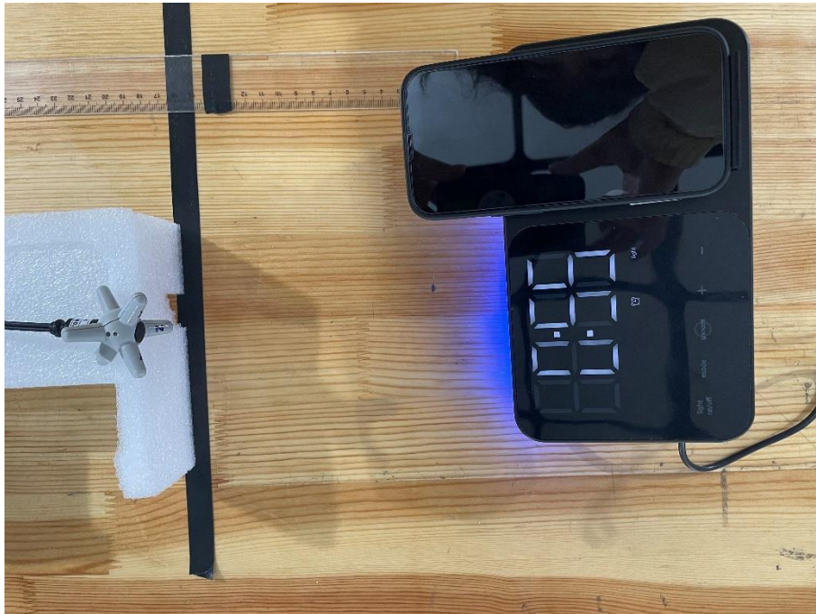
E-field Test Setup Photo of Position B(15cm)
