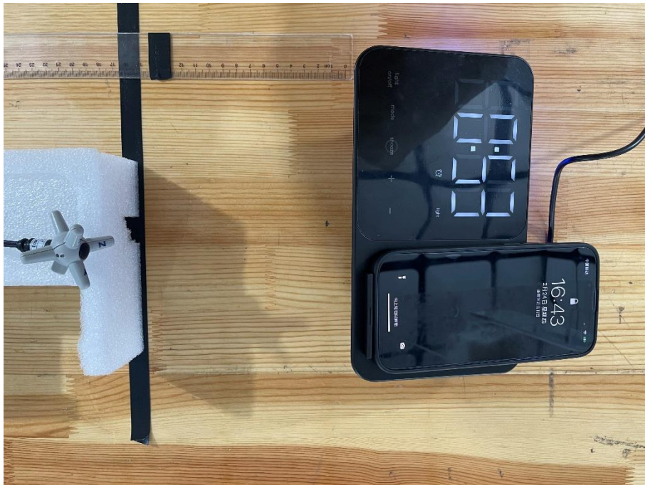
E-field Test Setup Photo of Position D(15cm)
