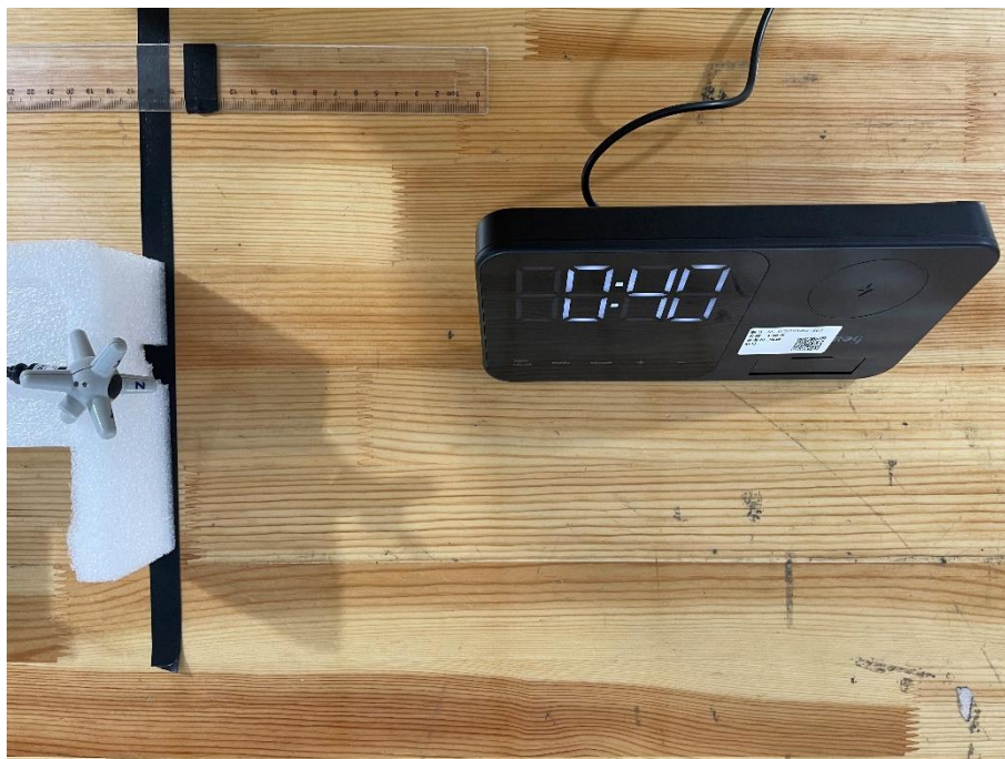
E-field Test Setup Photo of Position C(15cm)
