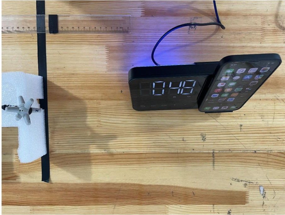
E-field Test Setup Photo of Position C(15cm)
