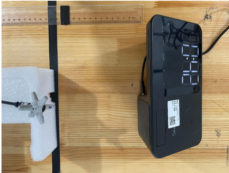
E-field Test Setup Photo of Position D(15cm)
