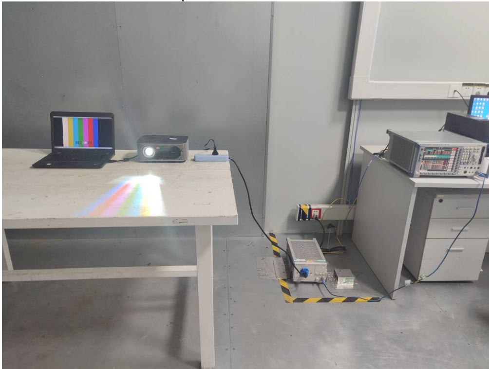
Photos of radiated emission test 30MHz – 1GHz
