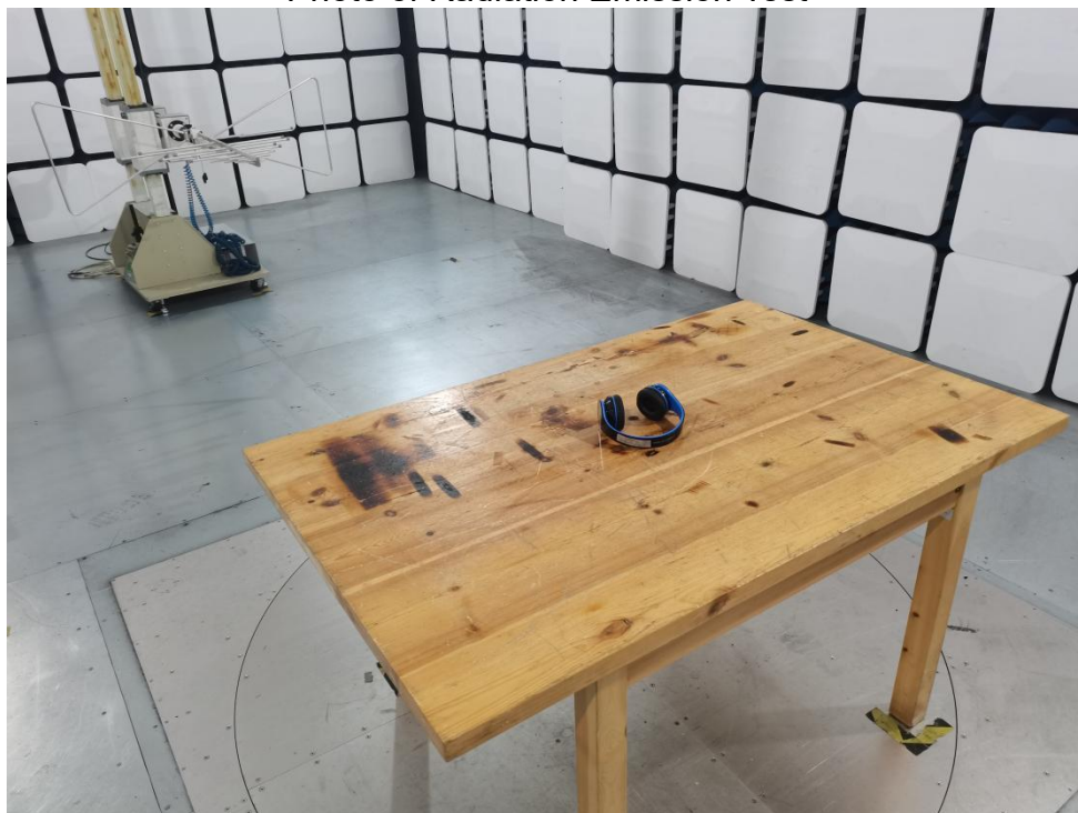
Photo of Radiation Emission Test
