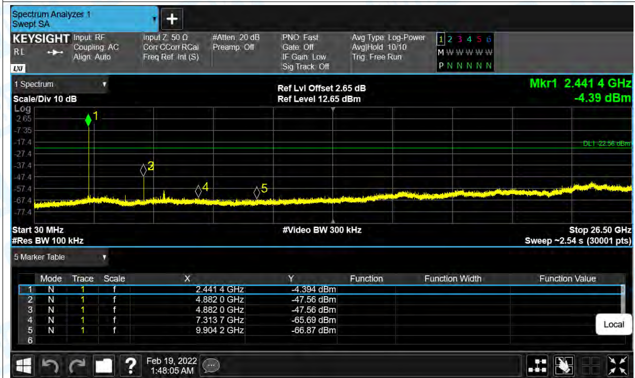
Tx. Spurious NVNT 1-DH1 2441MHz Ant1 Emission
