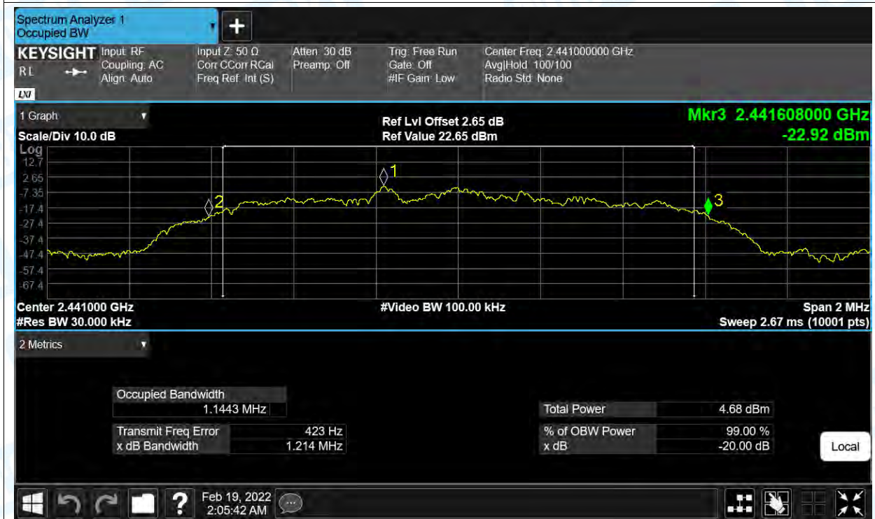
-20dB Bandwidth NVNT 3-DH1 2441MHz Ant1
