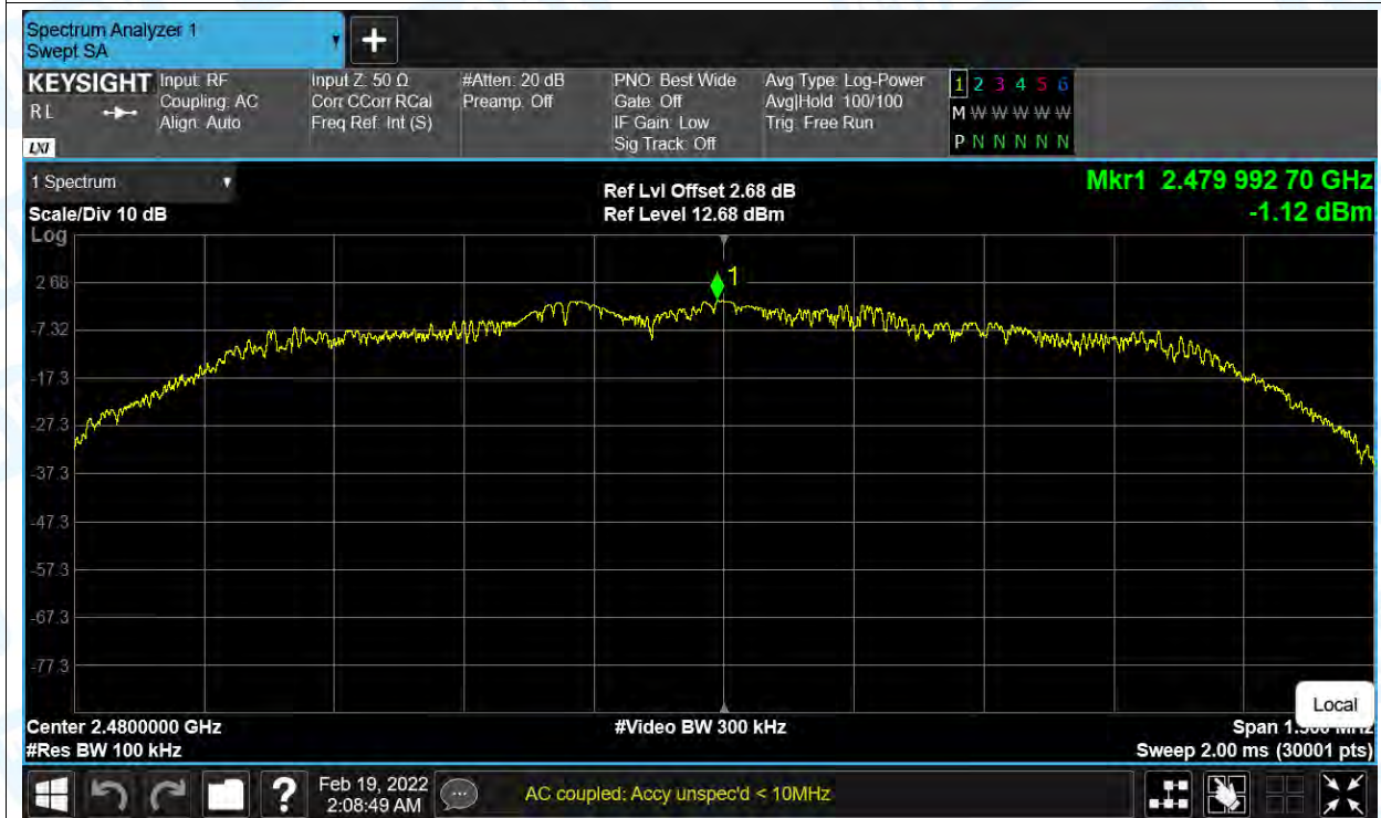
Tx. Spurious NVNT 3-DH1 2480MHz Ant1 Emission
