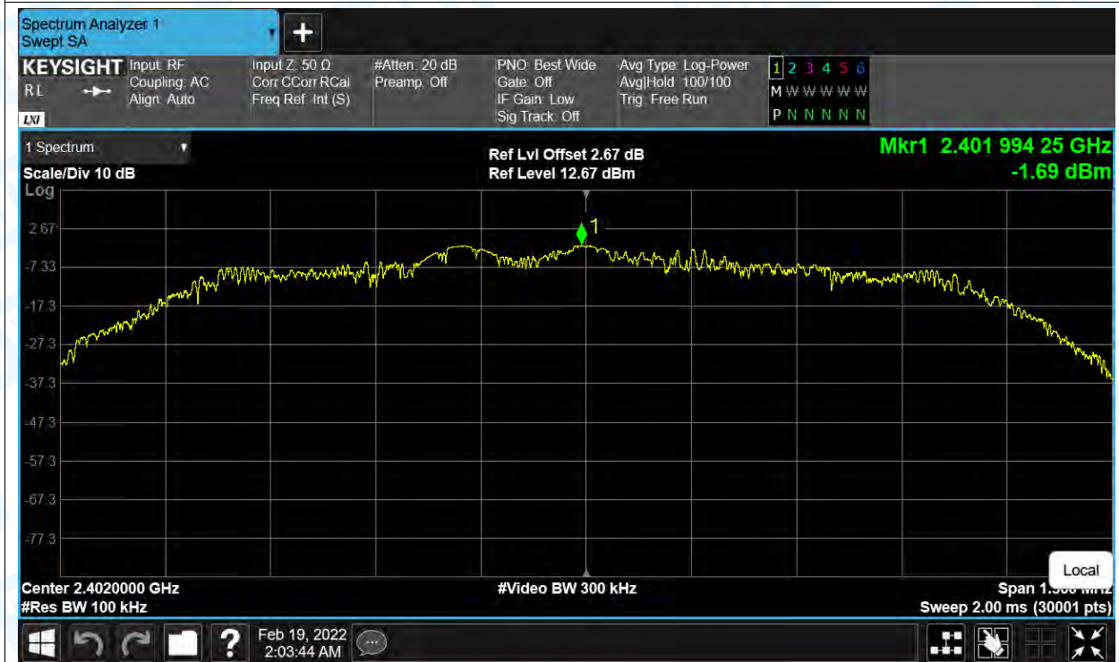
Tx. Spurious NVNT 3-DH1 2402MHz Ant1 Emission
