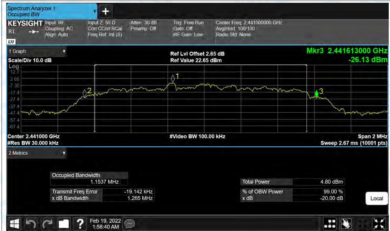
-20dB Bandwidth NVNT 2-DH1 2480MHz Ant1
