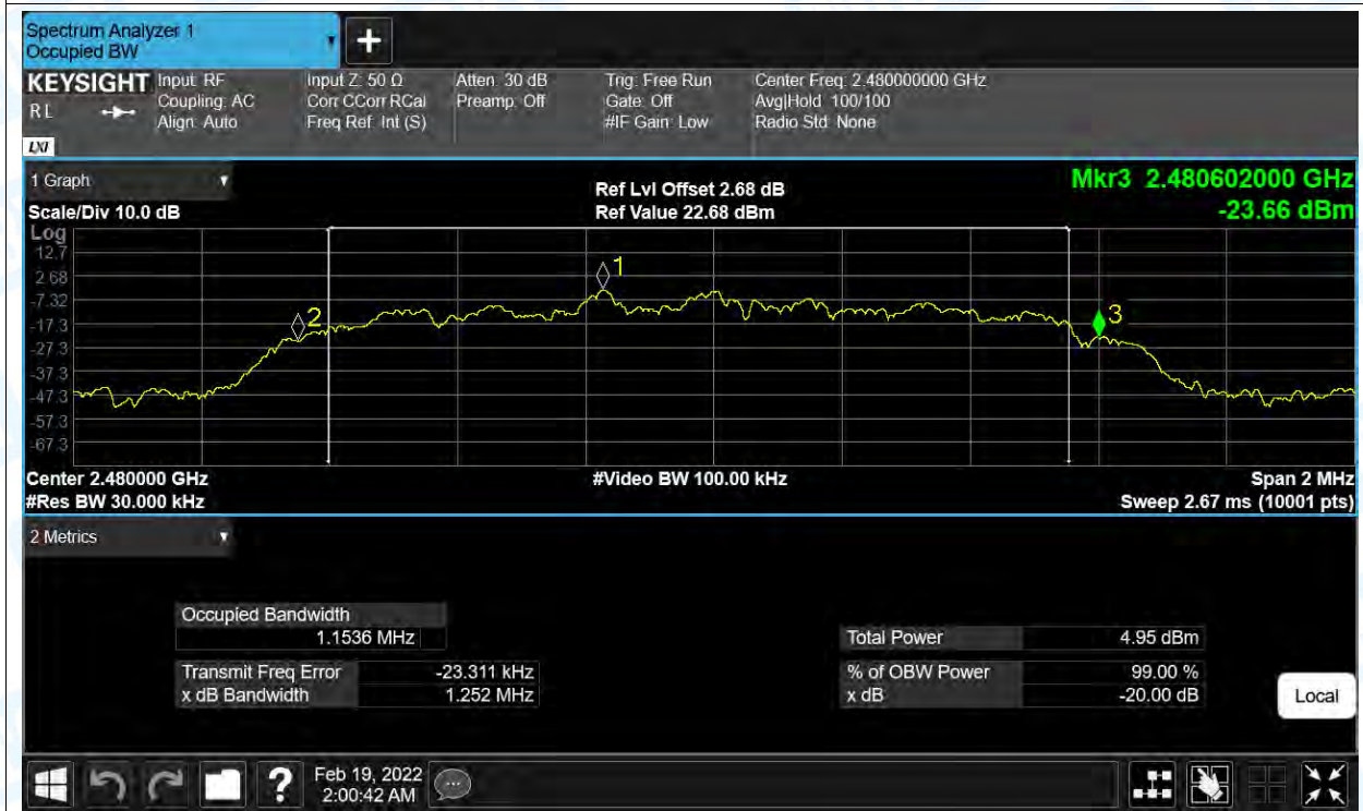
-20dB Bandwidth NVNT 2-DH1 2480MHz Ant1
