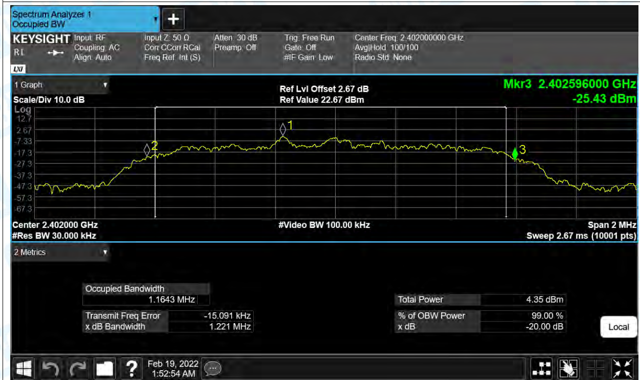
-20dB Bandwidth NVNT 2-DH1 2402MHz Ant1
