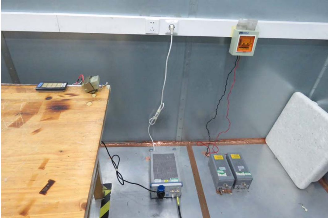
Picture 2 Conducted Emission Test Setup
